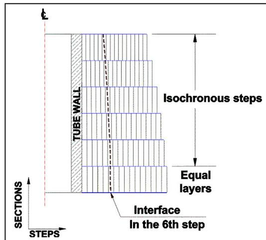
Figure 3. Geometry used in the computation
