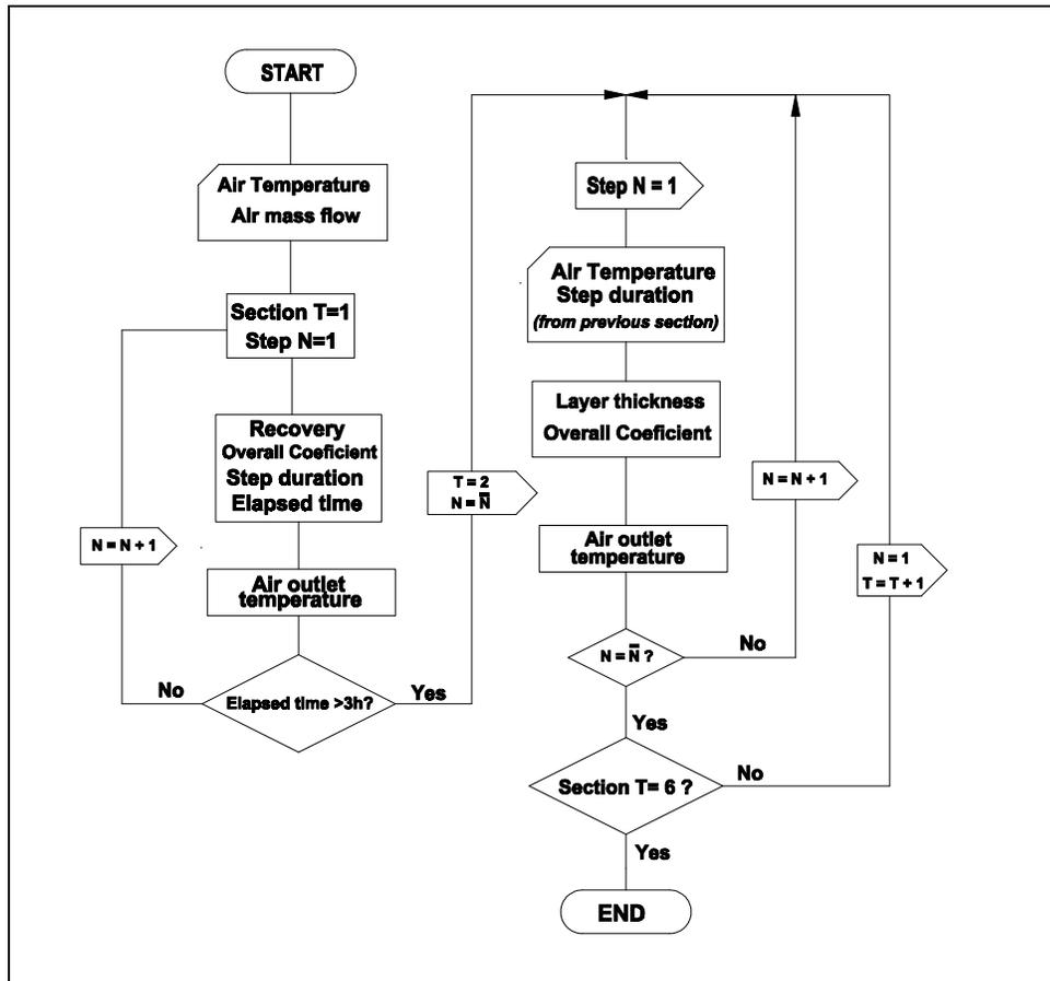
Figure 4. Logic diagram for the computation process
