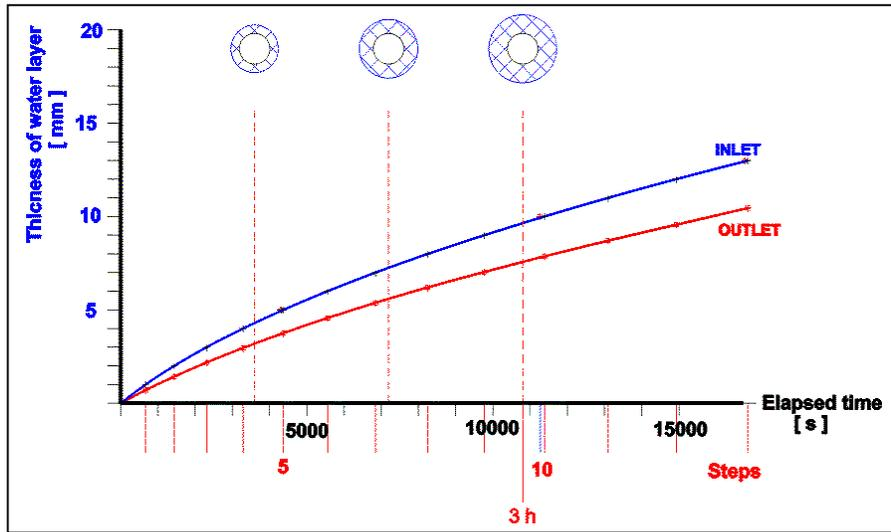
Figure 5. Progress of the molten layer thickness
