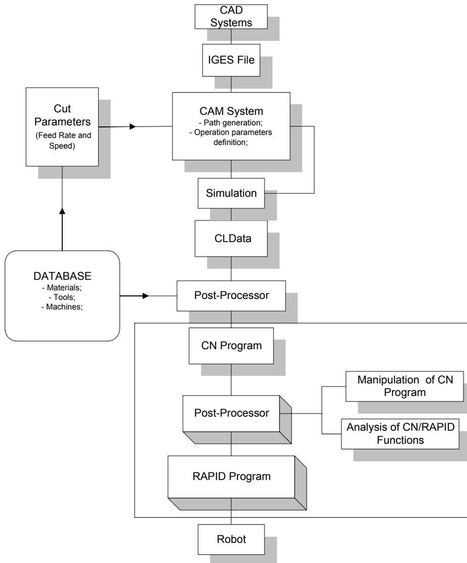
Figure 1. General structure of the Implemented System.
