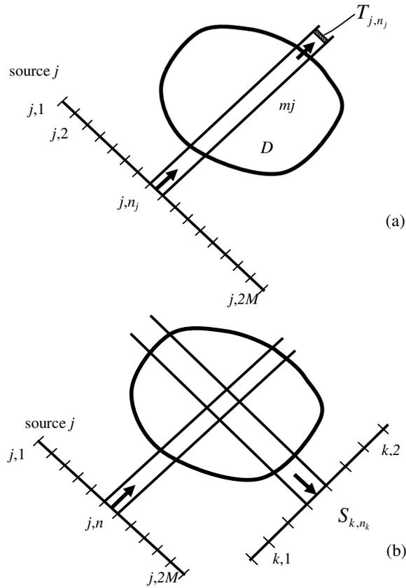
Figure 2- Two experiments used in the two steps approach (a) Experiment 1: Transmitted radiation measurement. (b) Experiment 2: Scattered radiation measurement.
