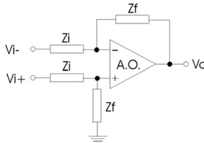
Figure 1. Generic configuration of a circuit with an operational amplifier.
