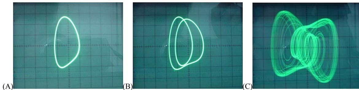
Figure 5. Phase-plane for forced Duffing system observed on oscilloscope (CH X = 1V/div and CH Y = 1V/div): (A)  $V_0=0.7$ ; (B)  $F_0=0.8$ ; (C)  $F_0=1.1$ .
