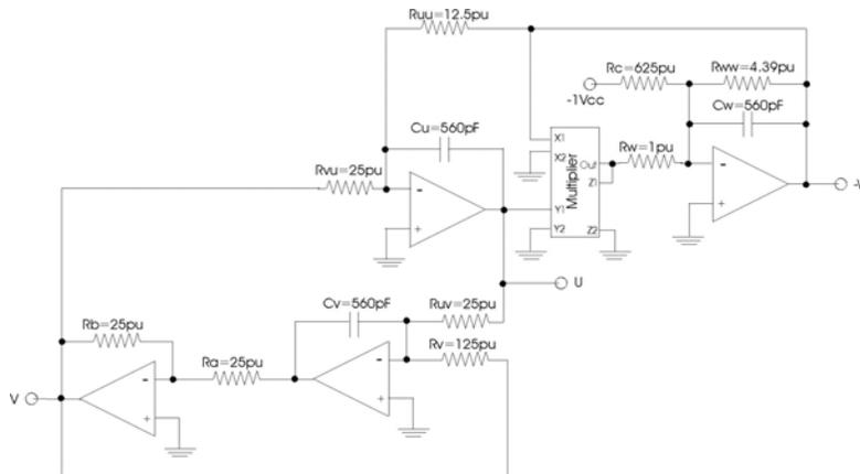
Figure 10. Rössler based chaotic circuit
