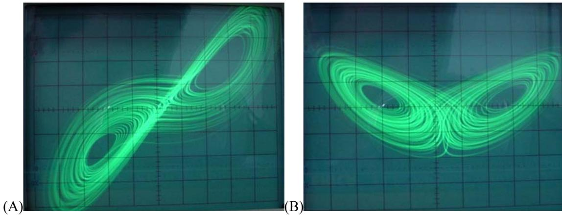
Figure 8. Chaotic Lorenz attractor observed on oscilloscope (CH X = 1V/div and CH Y = 1V/div): (A) projection on  $uv$ -plane; (B) projection on  $uw$ -plane
