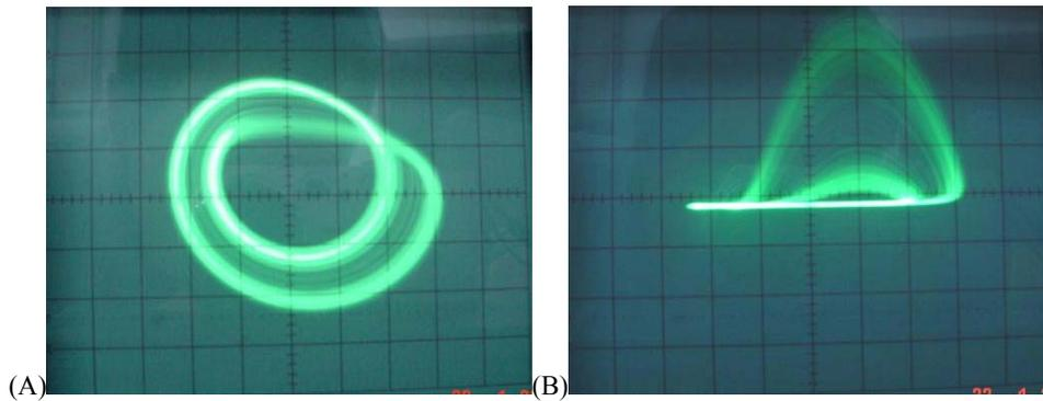
Figure 11. Rössler Band observed on oscilloscope (CH X = 2V/div and CH Y = 2V/div): (A) projection on  $uv$ -plane; (B) projection on  $uw$ -plane
