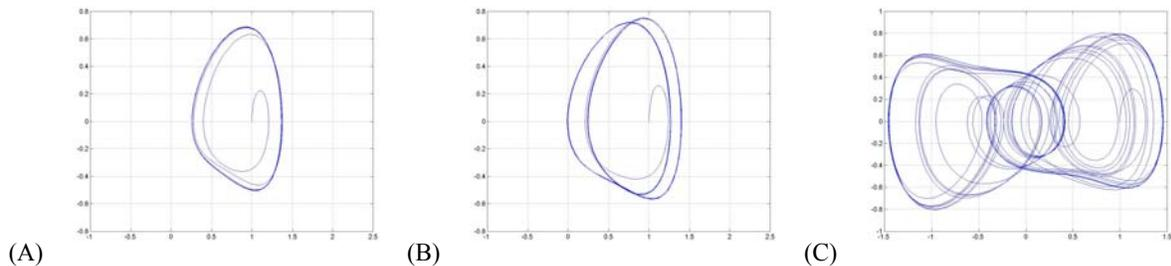
Figure 3. Phase-plane for forced Duffing system: (A)  $F_o=0.6$ ; (B)  $F_o=0.7$ ; (C)  $F_o=0.8$ .
