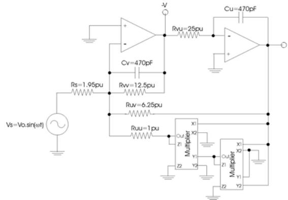
Figure 4. Forced Duffing based chaotic circuit
