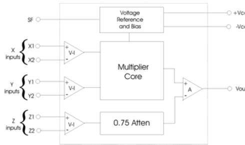
Figure 2. Schematic block diagram of an analog multiplier
