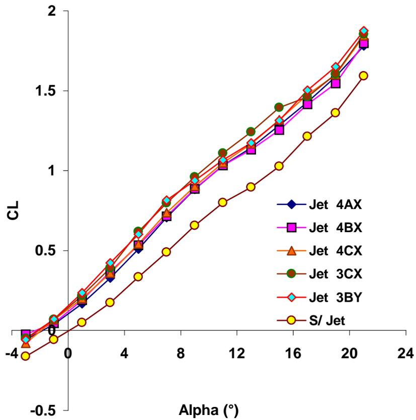
Figure 11 Lift curves for Triple Jets.
