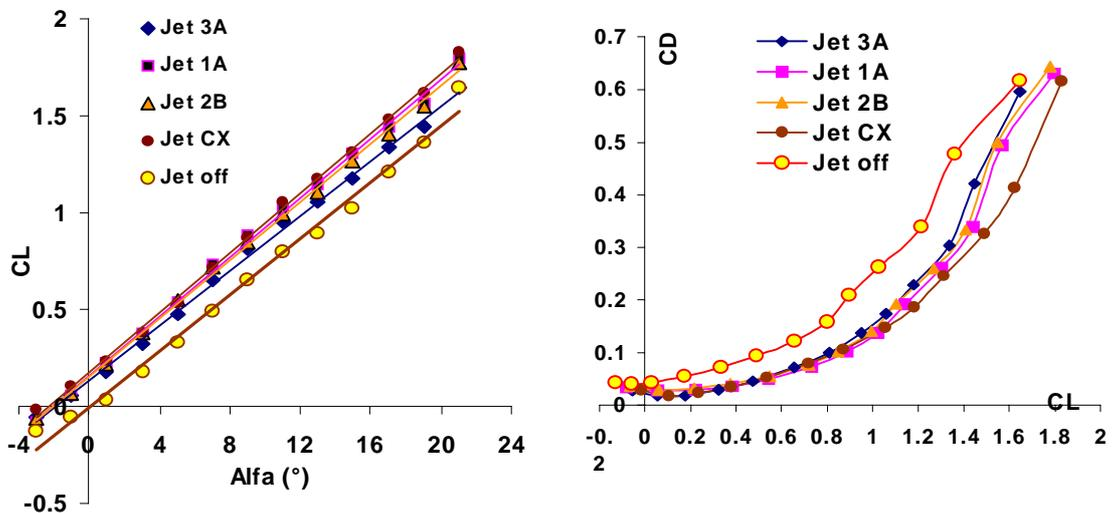
Figure 9 Double Jets Lift to alpha curves and Drag polar.
