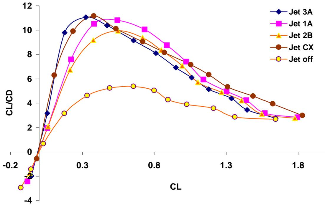
Figure 10 Wing efficiency with Double jets.
