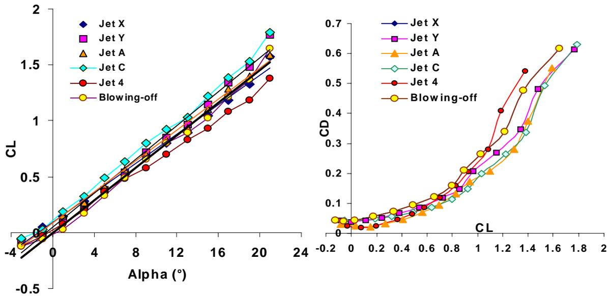
Figure 7 Single jet lift to alpha curves and Drag polar.
