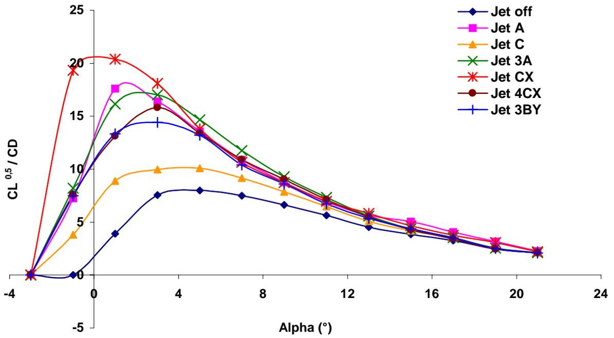
Figure 14 maximum range factor results of the best configurations.
