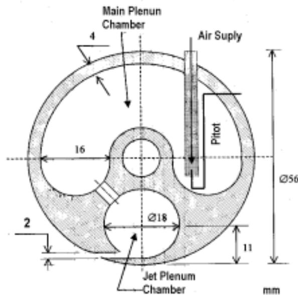
**Figure 3** Jet module geometry and dimensions.
