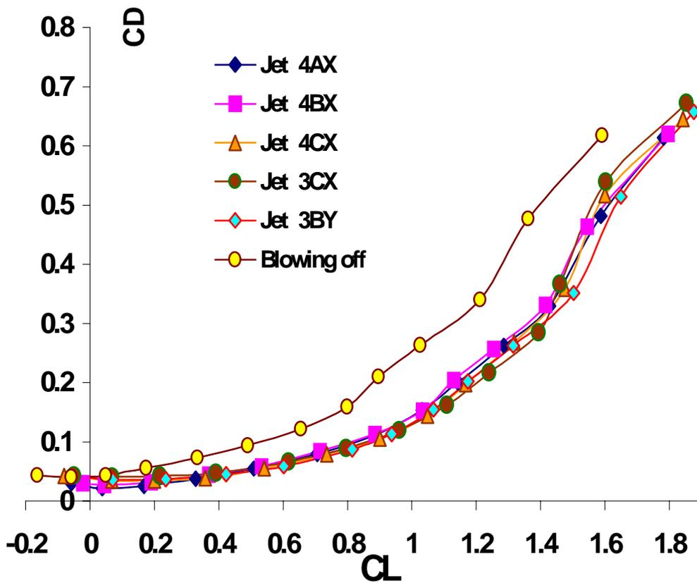
Figure 13 Drag polar for Triple Jets.
