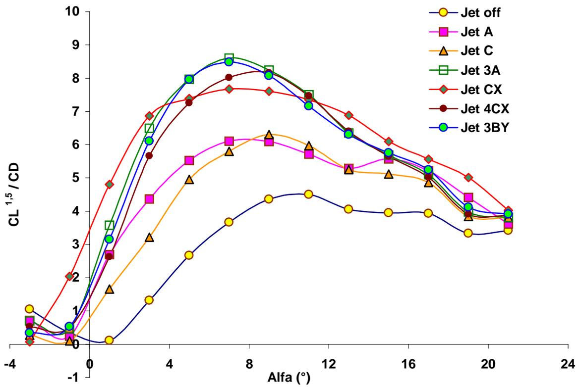
Figure 15 Climb rate factor results of the best configurations.
