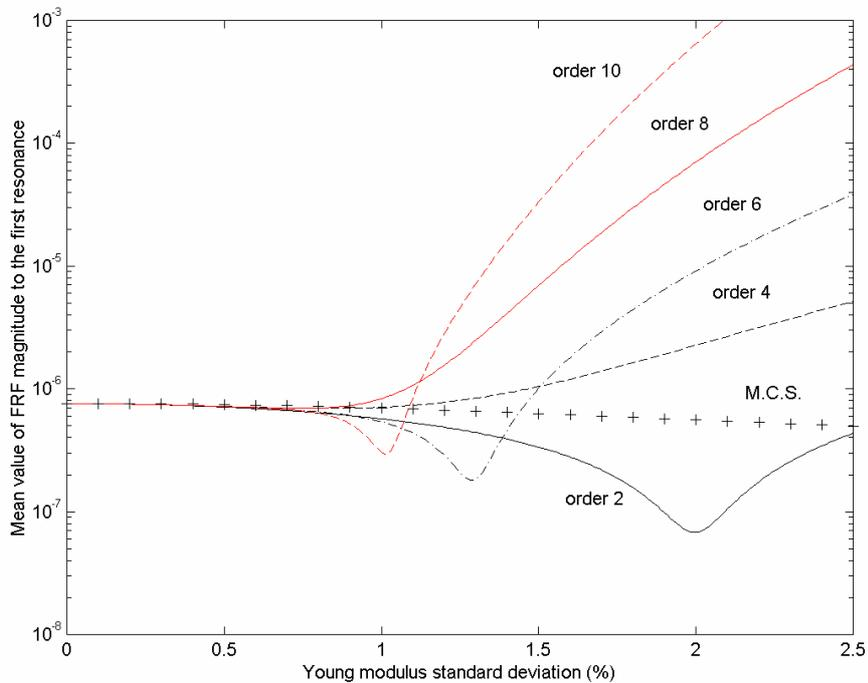
Figure 3: comparison of the mean value evolution in the interval  $[0; 2.5]$  – Young's modulus gaussian distribution case.
