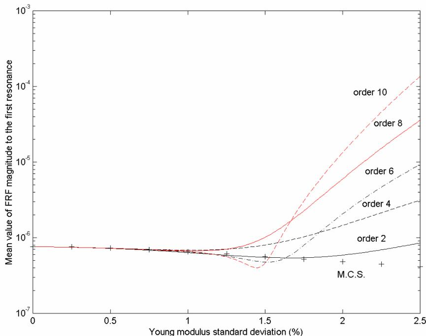
Figure 6: comparison of the mean value evolution in the interval [0; 2.5] – Young's modulus uniform distribution case.
