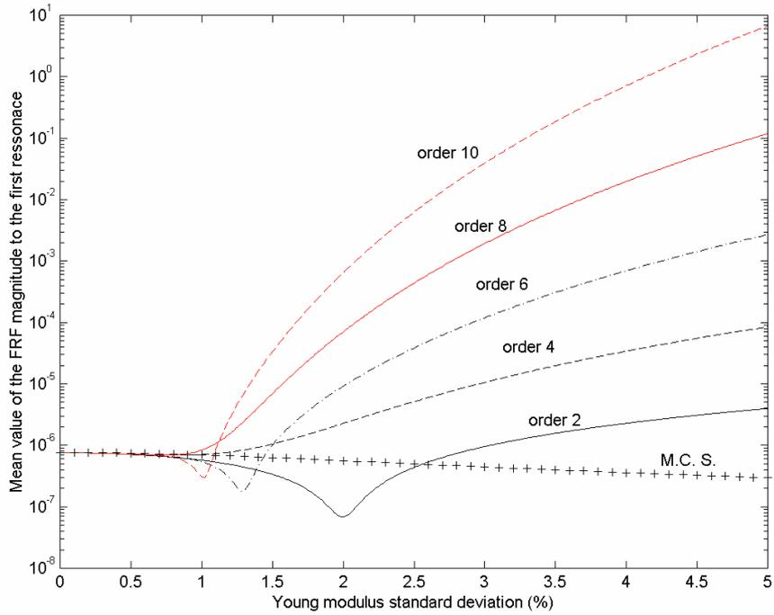
Figure 2: comparison of the mean value evolution in the case of a Young's modulus gaussian distribution.
