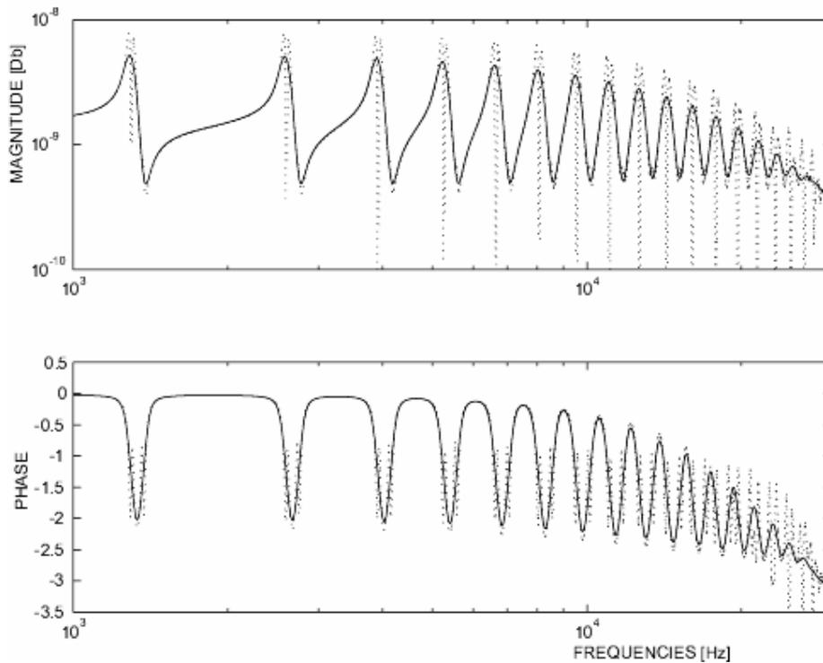
Figure 1. Mean FRF (magnitude and phase) - Monte Carlo simulation ( — ) and Perturbation method ( ..... ).
