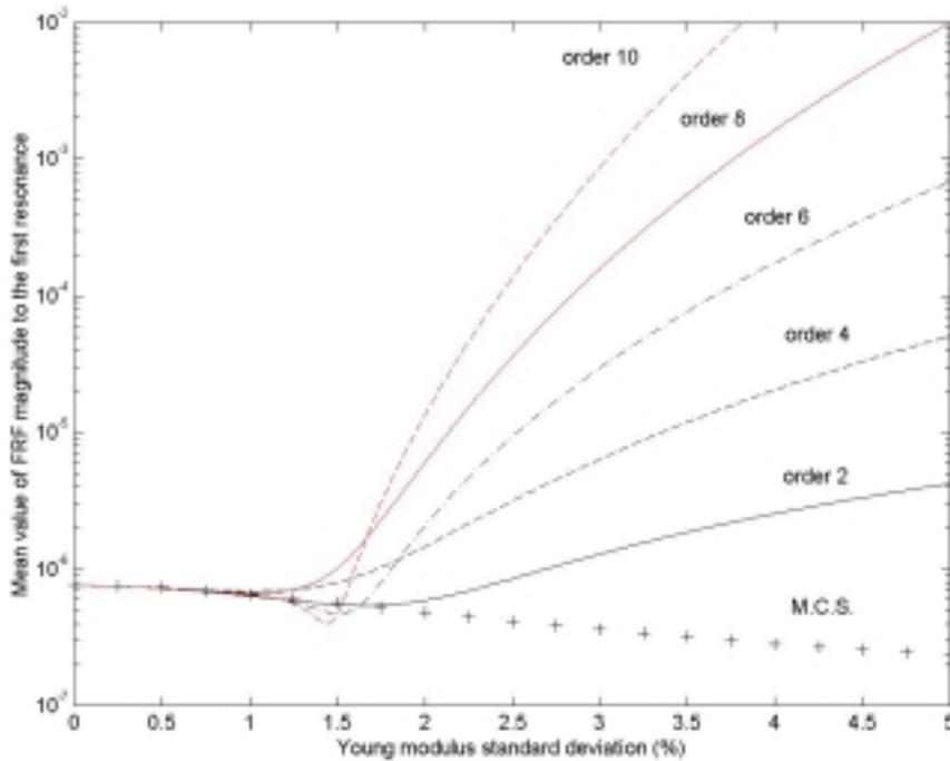
Figure 5: mean value evolution comparison in the case of a Young's modulus uniform distribution
