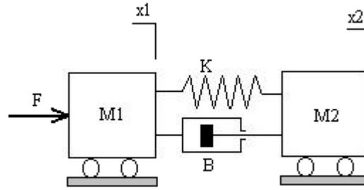
Figure 3. Mass-spring-damper model of the spindle
