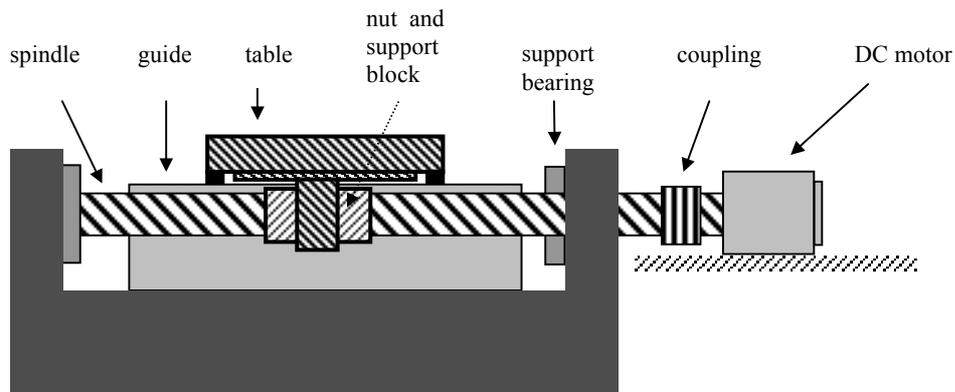
Figure 2. Principal components of the axis
