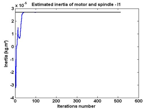
Figure (12) – Recursive estimation of motor inertia
