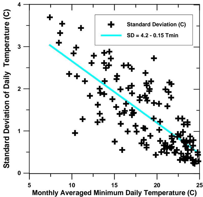
Figure 1. Dependence on the monthly averaged minimum daily temperature of the standard deviation of daily mean ambient temperature to the monthly mean ambient temperature, for 108 months in 9 cities.
