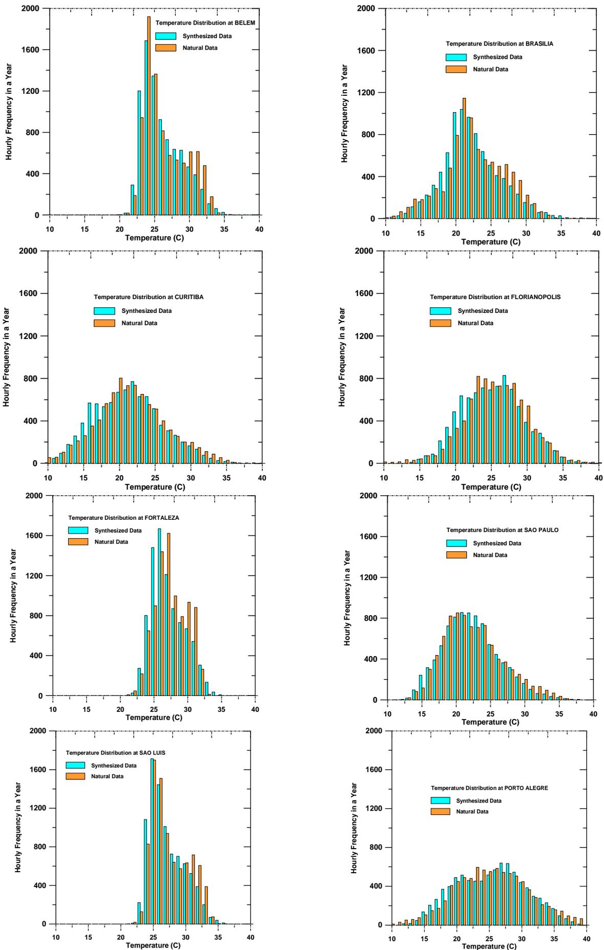
Figure 9 Comparison of the frequency of the hourly temperatures along a year for 8 cities in Brazil. Green bars are frequencies from synthesized data and orange bars are frequencies from natural data (TRY files).
