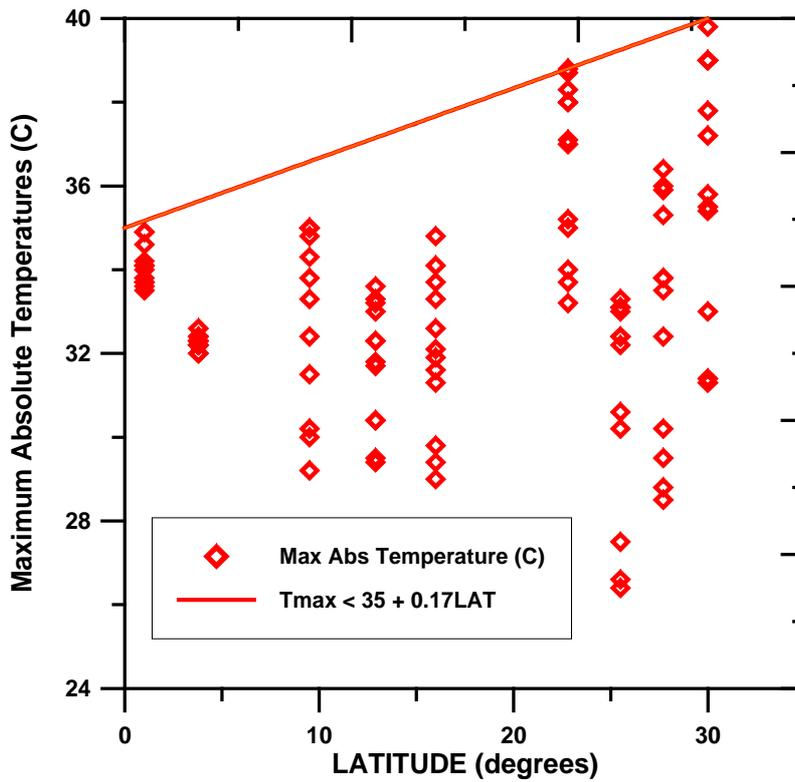
Figure 4. Maximum absolute ambient temperature for each month plotted in function of the site latitude. The straight line represents an equation used for limiting the generated temperatures in each day
