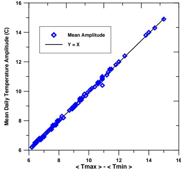
Figure 5. Linear correlation between the mean daily temperature amplitude and the difference between the monthly averaged maximum temperatures and the monthly averaged minimum temperatures
