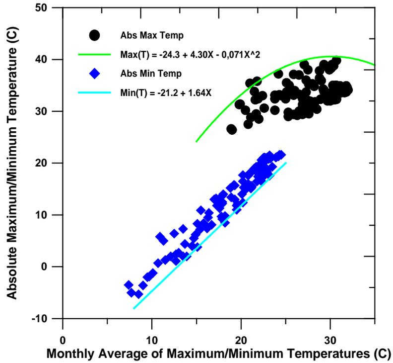
Figure 3. Values of the absolute maximum temperature (black dots) plotted in function of the monthly average of the daily maximum temperature and values of the absolute minimum temperature (blue dots) plotted in function of the monthly average of the daily minimum temperature. The lines represent equations used for limiting the generated temperatures in each day.
