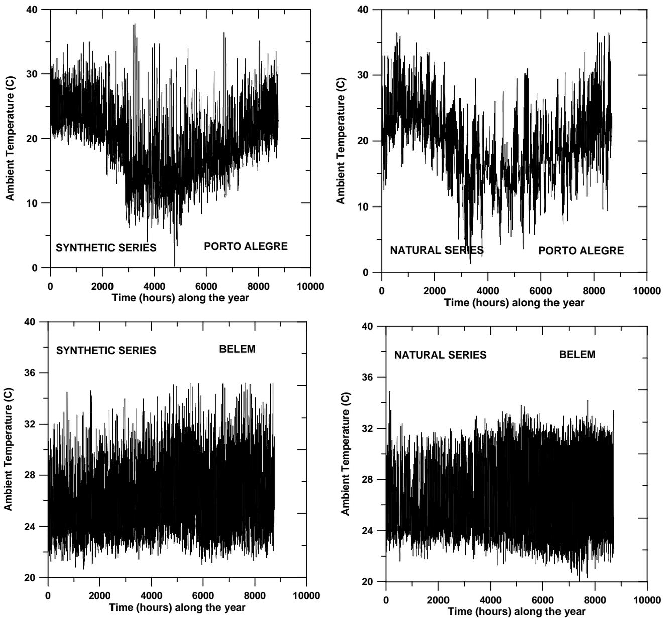
Figure 7. Temperature profiles for Porto Alegre and Belém as synthesized with the presented algorithm (left) and respective natural profiles as recorded in TRY files (right).
