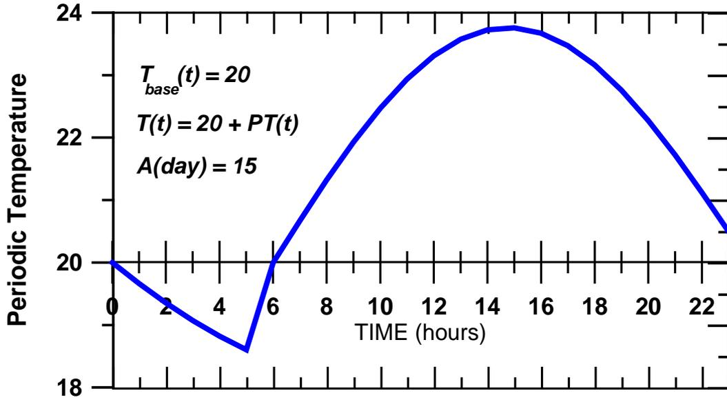
Figure 6. Periodic function used to determine the periodic term in the temperature synthesizing. In this example the base temperature remain constant  $T_{base}(t) = 20^{\circ}\text{C}$  and the temperature amplitude was considered  $A(day) = 15^{\circ}\text{C}$ .
