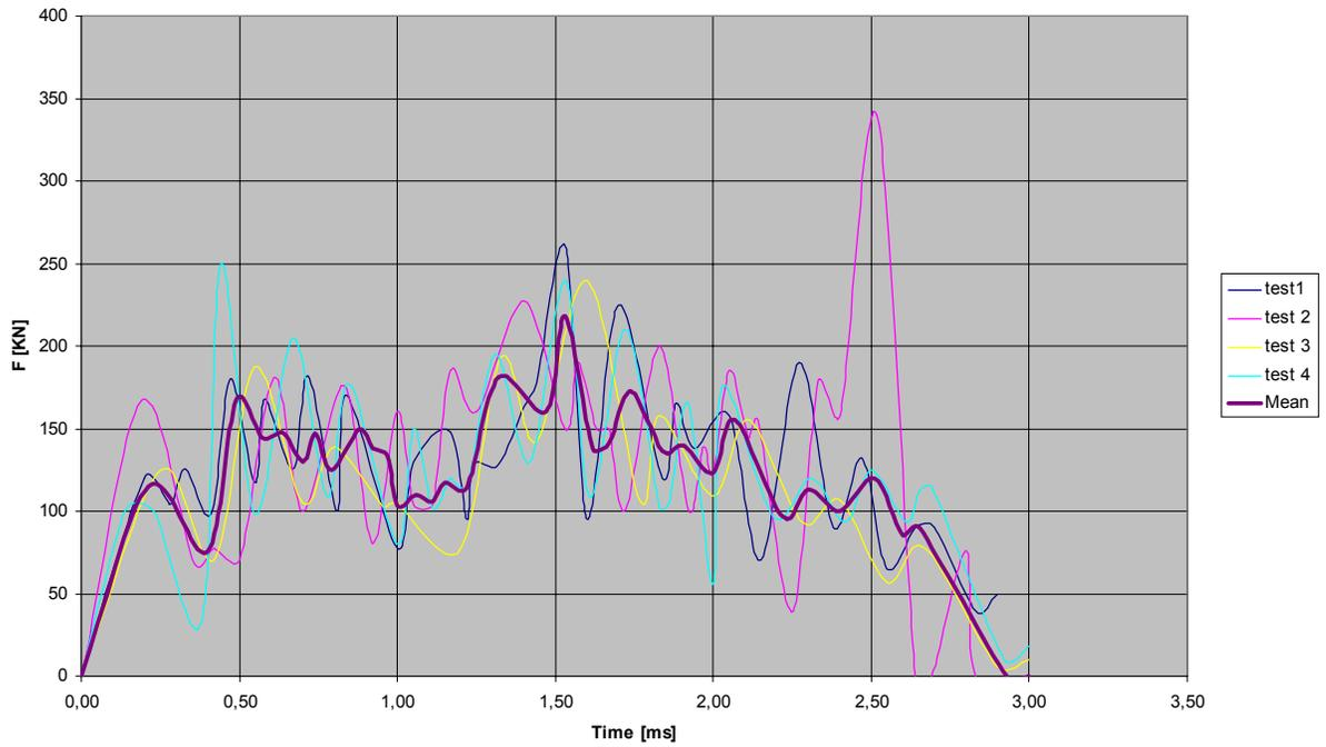
Figure 8: Recorded reactions at missile-target interface for tested projectiles
