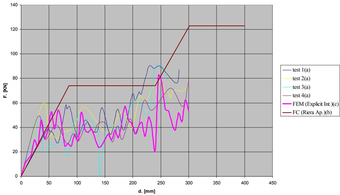
Figure 6: Numerical predictions and experimental results for static crushing load.
