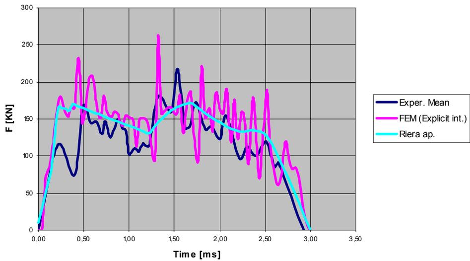
Figure 9: Comparison between experimental and numerical results for the reaction vs. time function at the projectile-target interface.
