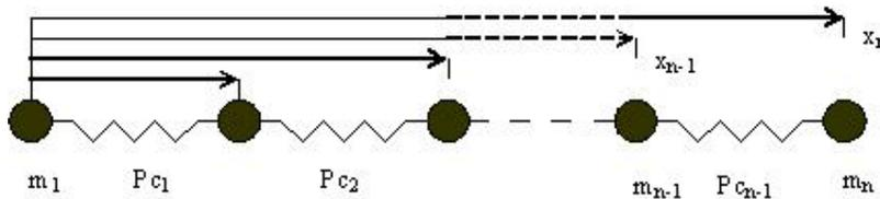
Figure 3: Discrete Model of projectile (Model 1)
