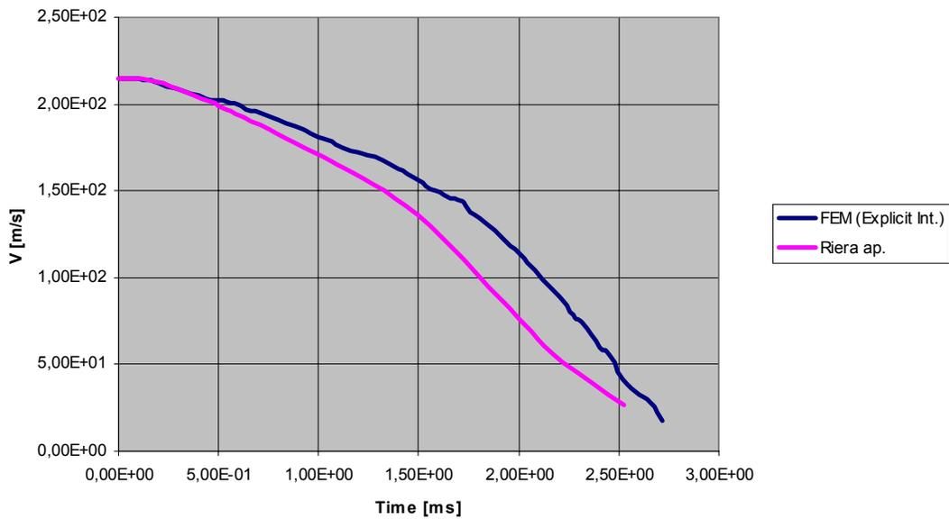
Figure 11: Residual velocity vs time for Models 1 and 2.
