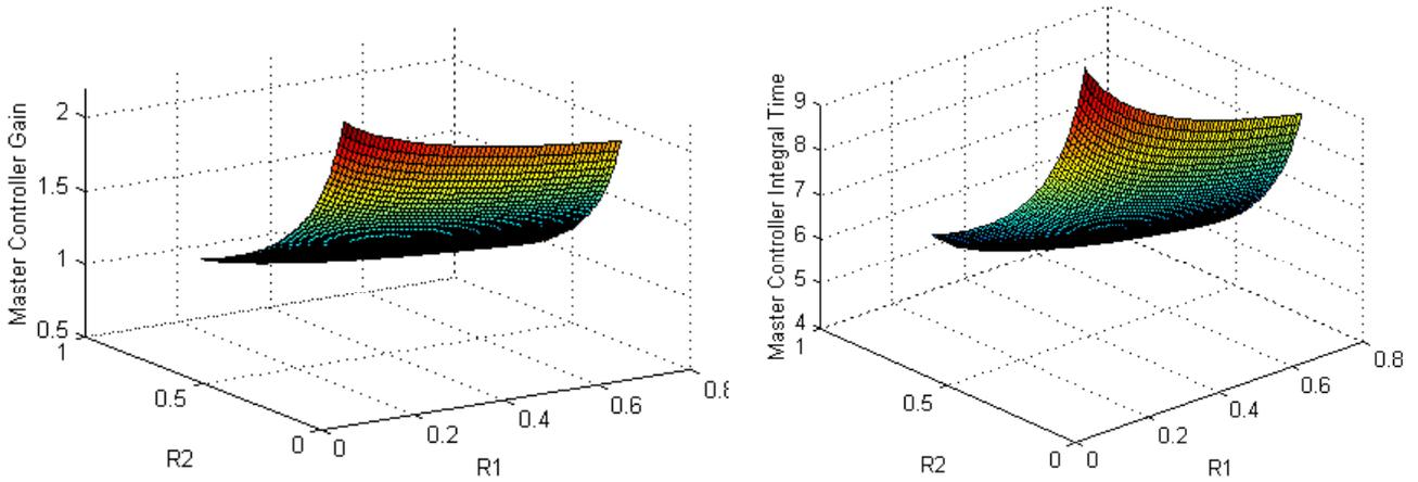
Figure 3. Response surfaces for master controller proportional gain and master controller integral time based on the tuning equations set found to PI-PI cascade architecture.
