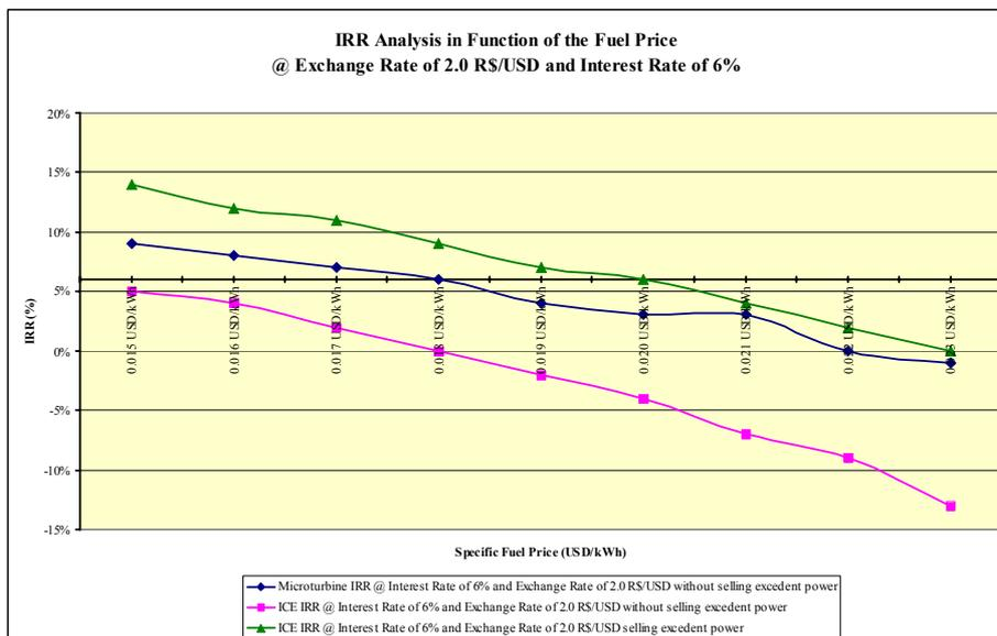
Figure 8 – IRR analysis in function of the specific fuel cost for an interest rate of 6% p.a. as datum.
