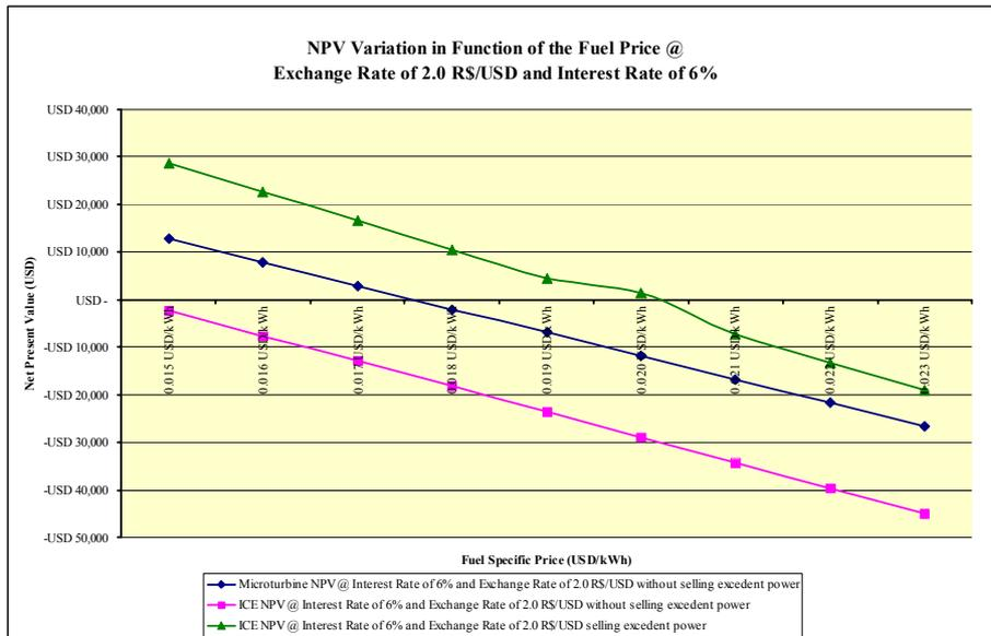
Figure 7 – NPV analysis in function of the specific fuel cost (condition 5).
