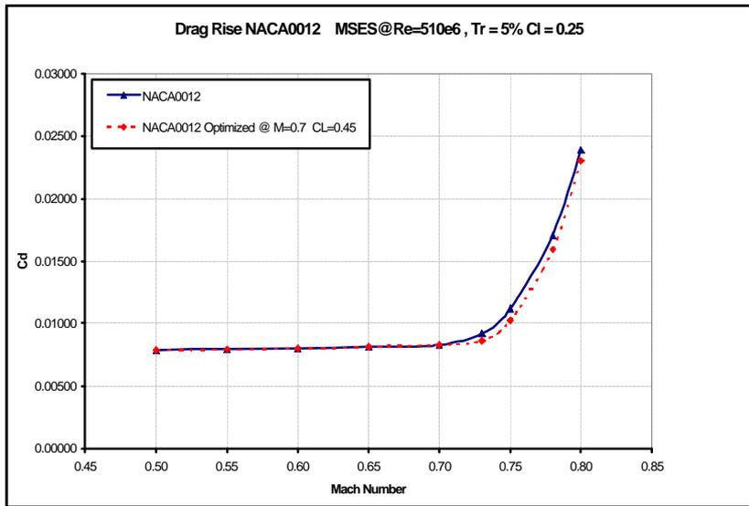
Figure 6. Optimized NACA0012 airfoil evaluated for  $Cl=0.25$ .
