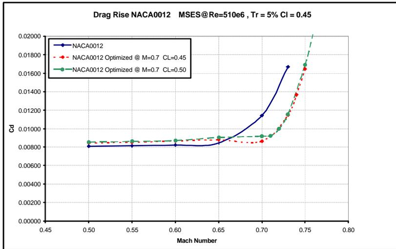
Figure 7. Comparison of the drag rise curves between different optimized NACA0012 airfoils evaluated at  $Cl=0.45$ .
