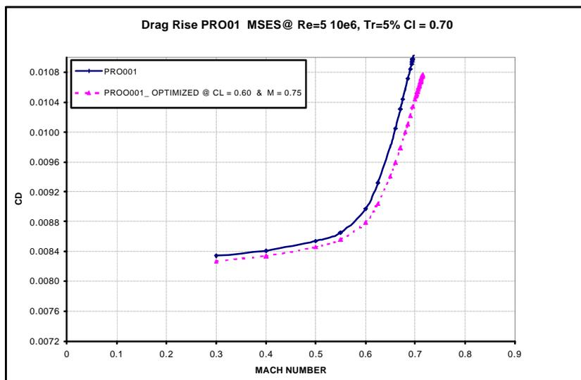
Figure 11. Drag rise curves for the original and optimized PRO01 airfoils at  $Cl=0.70$ .
