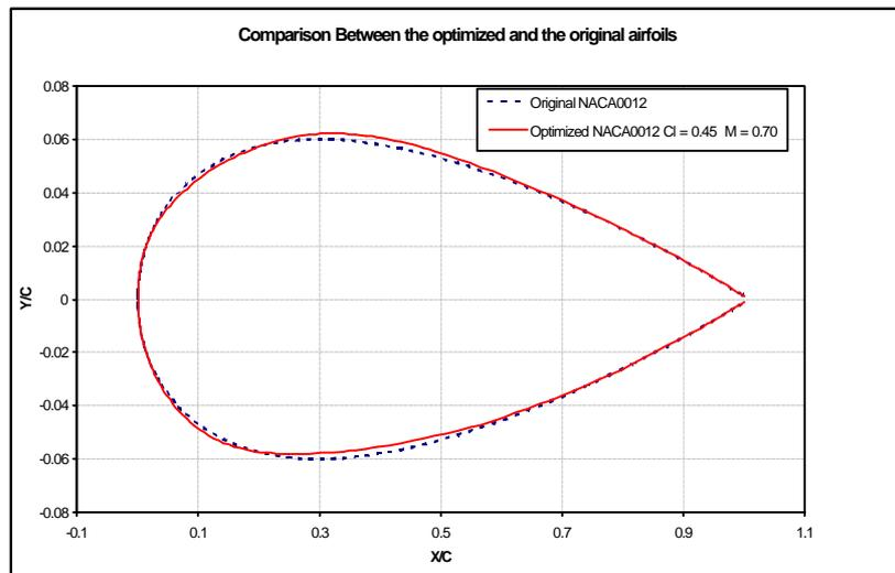
Figure 3. Comparison between the optimized and the original airfoil.
