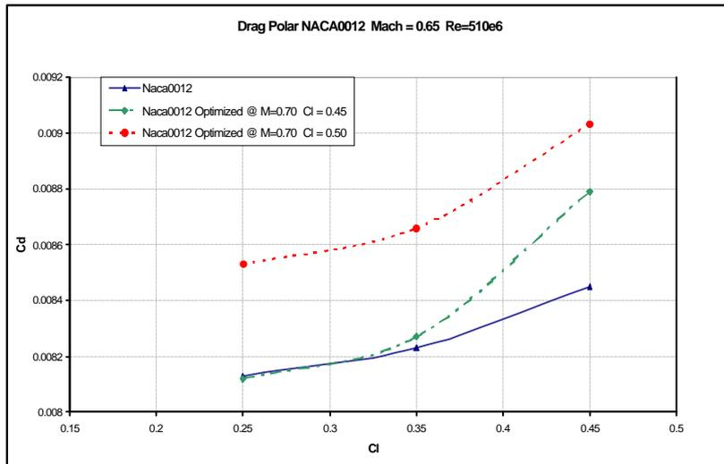
Figure 10. Drag polar curves for original and optimized NACA0012 airfoils at Mach number of 0.65.
