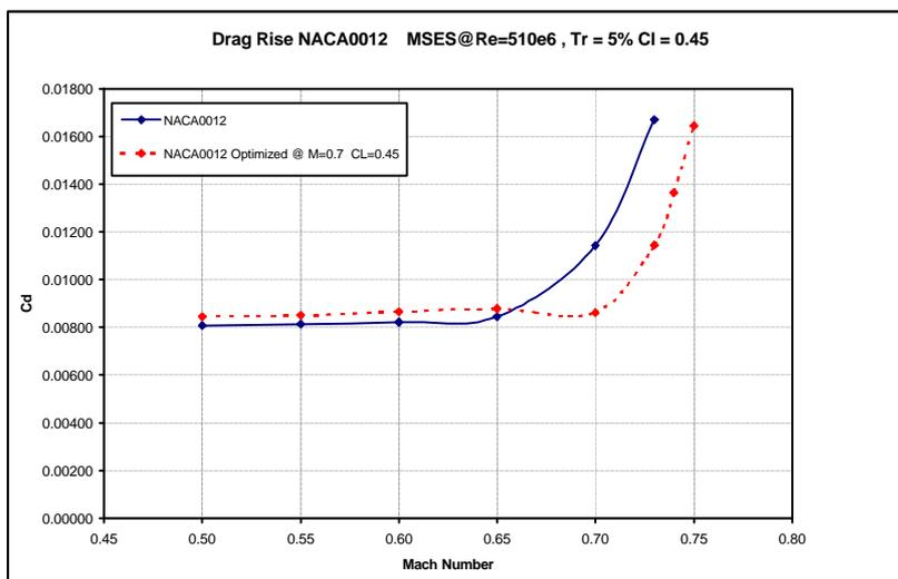
Figure 4. Drag rise evaluation for the optimized NACA0012 airfoil.
