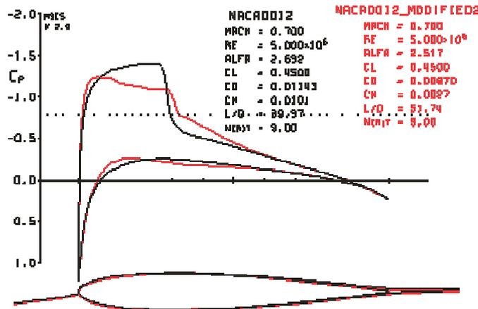
Figure 2. Comparison between the original NACA0012 airfoil and the optimized airfoil.
