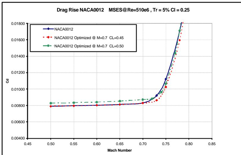
Figure 8. Drag rise curves for the optimized NACA0012 airfoils evaluated at  $Cl=0.25$ .
