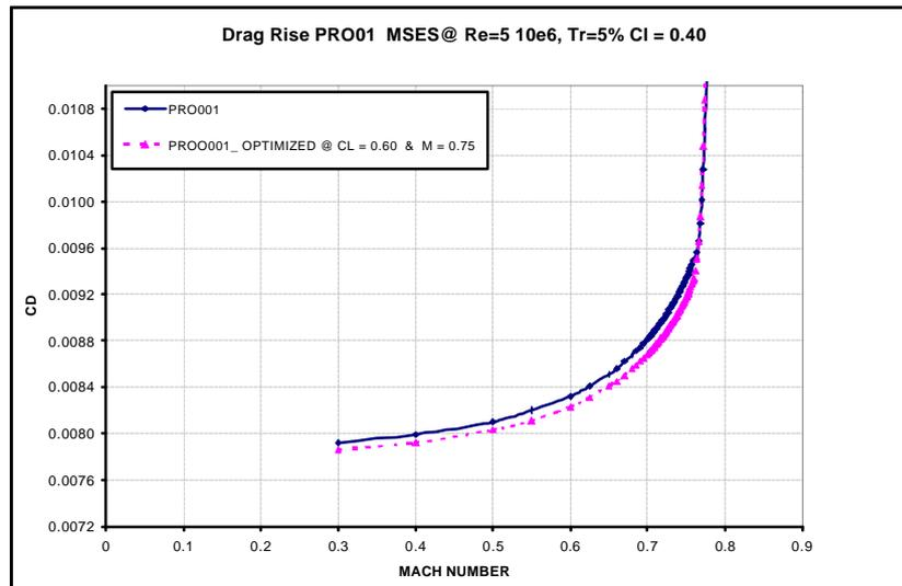
Figure 12. Drag rise curves for original and optimized PRO01 airfoils at  $Cl=0.40$ .
