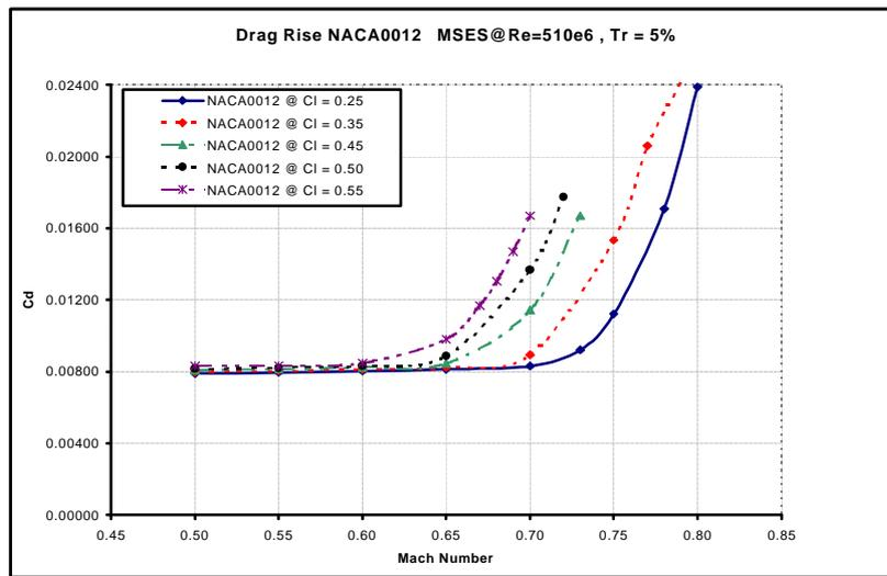
Figure 1. NACA0012 drag rise curves for a set of Cl values.
