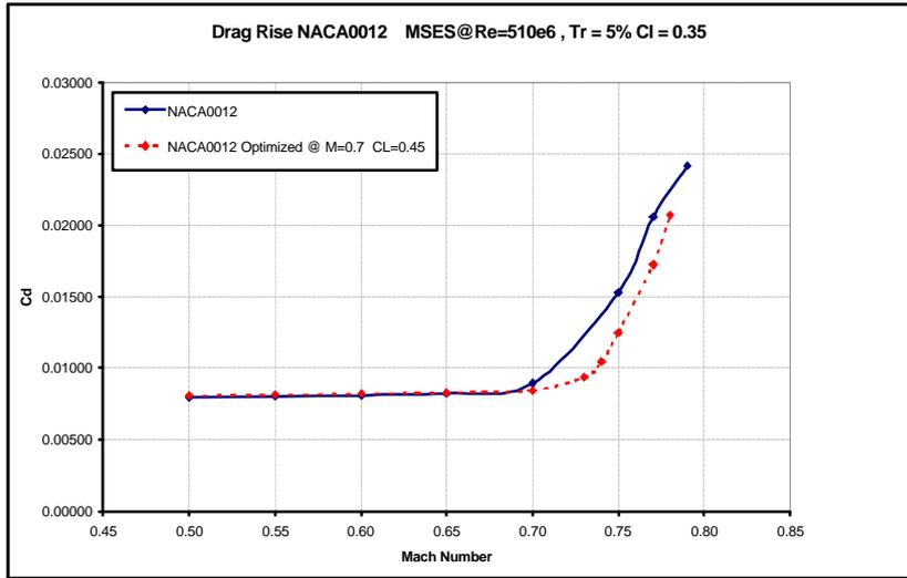
Figure 5. Optimized NACA0012 airfoil evaluated for  $Cl=0.35$ .
