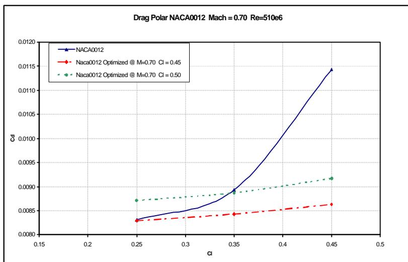
Figure 9. Drag polar curves for original and optimized NACA0012 airfoils at Mach number of 0.70.
