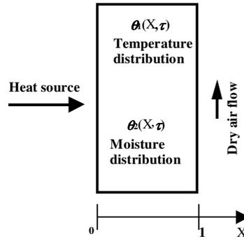
Figure 1 – Drying process schematic representation
