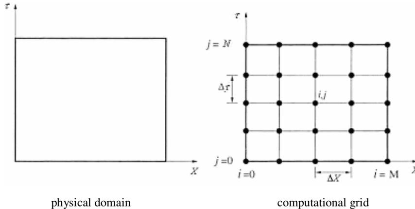
Figure 2 – Physical domain and computational grid
