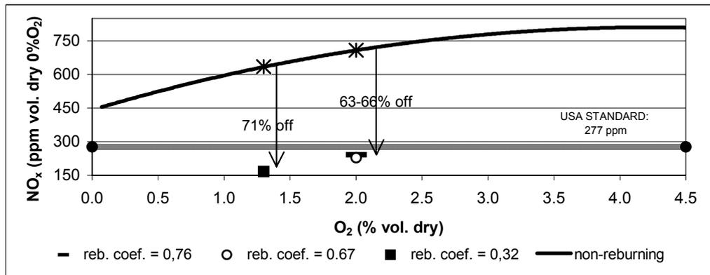
Figure 7. Effect of reburning on NO<sub>x</sub> emissions
