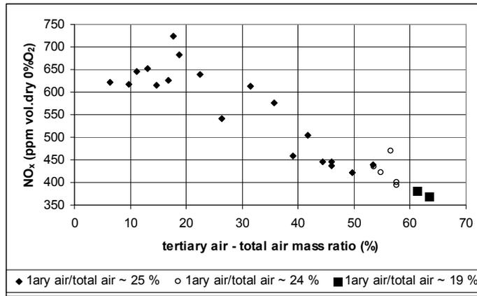
Figure 9. NO<sub>x</sub> emissions versus 3<sup>ary</sup> air - total air ratio
