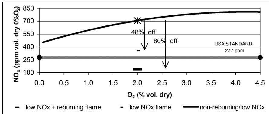
Figure 10. Effect of low NO<sub>x</sub> burner and low NO<sub>x</sub> burner + reburning on NO<sub>x</sub> emissions
