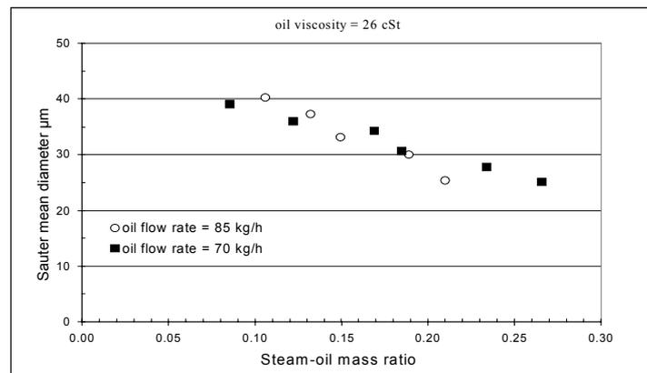
Figure 2. Droplet diameter versus atomization steam-oil ratio
