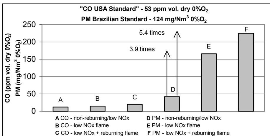
Figure 11. Effect of low NO<sub>x</sub> burner and low NO<sub>x</sub> burner + reburning on CO and PM emissions
