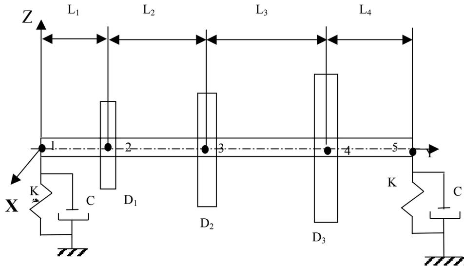
Figure 2 Multi disk rotor simulated
