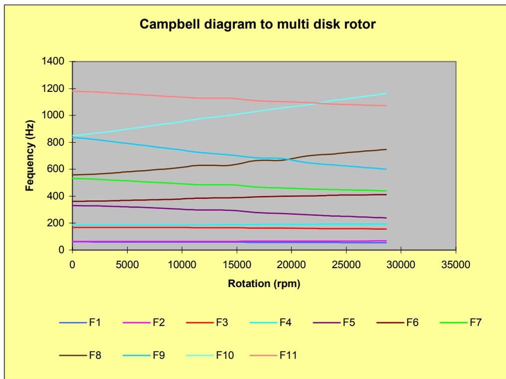
Figure 4 Campbell diagram to multi disk rotor
