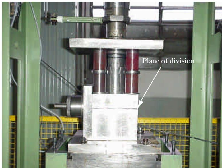
Figure 4. Hydroforming tools in the hydraulic press.
