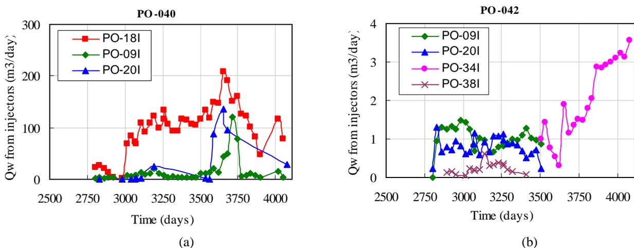
Figure 7. Water rate from injectors to producer PO-040 (a) and PO-042 (b)
