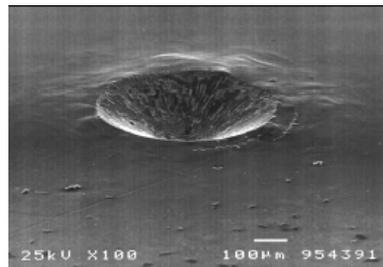
Figure 2. Plastic deformation of the substrate (Pile-up) taking place and extending approximately one indent diameter away from the edge of the indent (Thomsen et al 1998).
