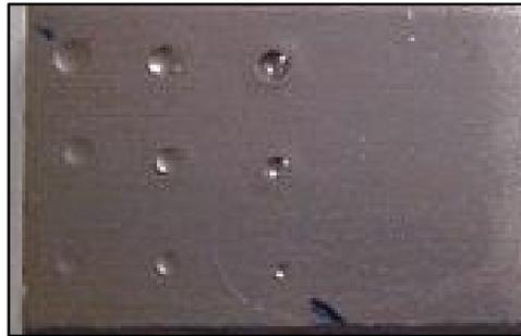
Figure 5. Indentation marks generated in the coated system during indentation with three spheres (Diameters of 6.3, 3.2, 1.59 mm) and three load levels (196.1, 294.2, 490.3 N).
