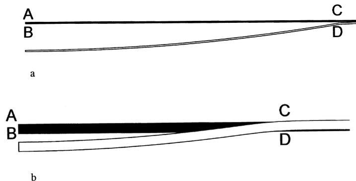
Figure 10 Bending of the film. FEM results obtained during the 50 N normal indentation of a system with different wear resistant films and an elastic-plastic 6061 aluminum substrate. Original (black) and displaced (white); (a) Thickness  $t = 0.6 \mu\text{m}$  and (b) Thickness  $t = 4.6 \mu\text{m}$  (Souza, 1999).
