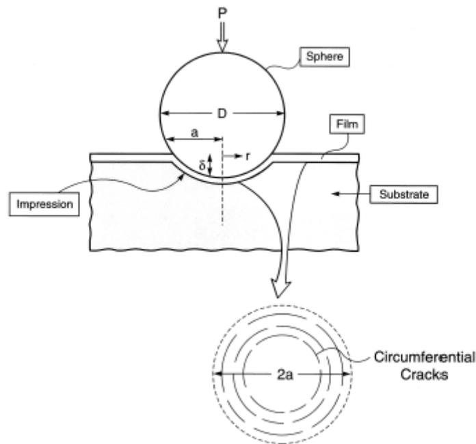
Figure 1. Representation of indentation model and circular cracks generated in the inside of the indentation zone (Begley et al 1999).
