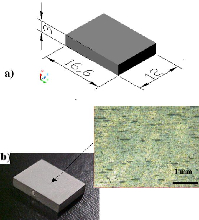
Figure 3. Coated system CrN-Aluminum. a) Specimen dimensions in milimeters b) Superficial aspect of the CrN coating obtained through a commercial PVD process.
