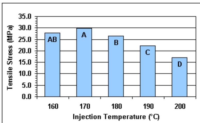
Figure 1. Mean tensile stress values at different temperatures.
