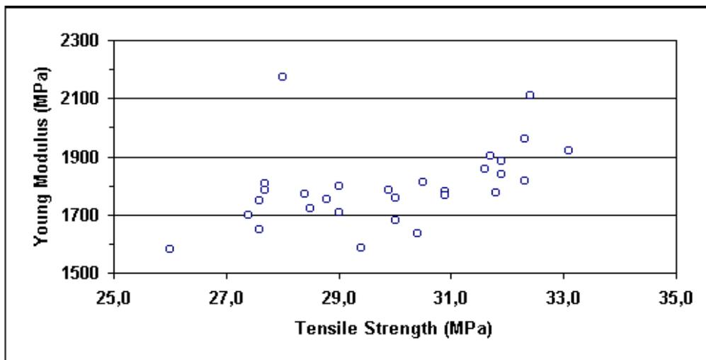
Figure 5. Dispersion diagram correlating Young Modulus and Tensile Strength at 170 °C.
