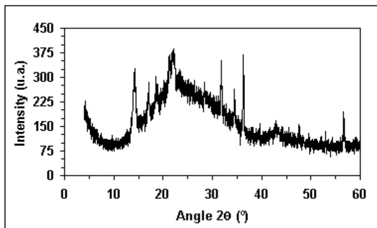
Figure 3. Polypropylene X-Ray analysis – Injection temperature = 160 °C.
