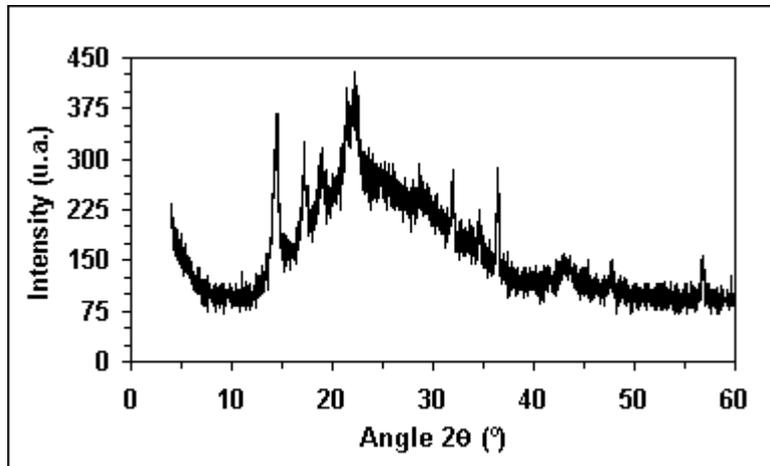
Figure 4. Polypropylene X-Ray analysis – Injection temperature = 160 °C.
