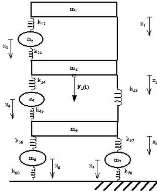
Figure 1. 7 d.o.f. mechanical system
