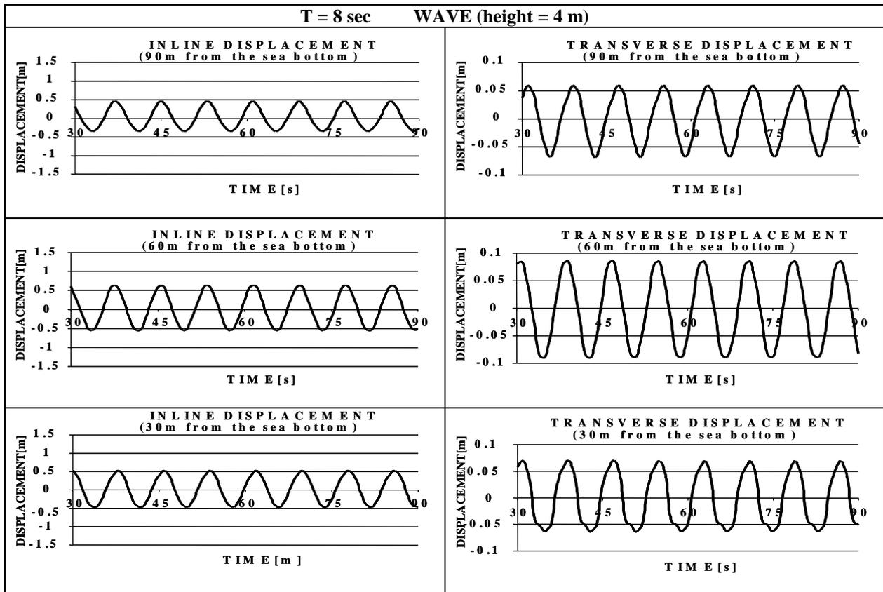
Figure 6. Riser inline and transverse displacements from simulations for three different locations along the riser for wave excitation with 8 seconds wave period.
