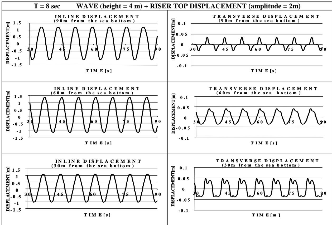
Figure 5. Riser inline and transverse displacements from simulations for three different locations along the riser for combined top displacement and wave excitations with 8 seconds wave period.
