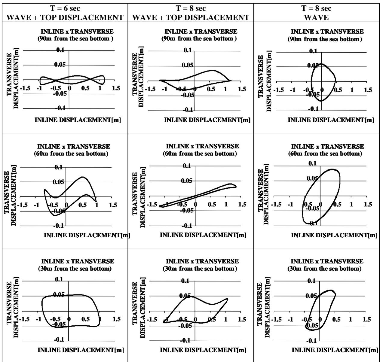
Figure 7. Riser planar displacements from simulations for the three different locations along the riser.
