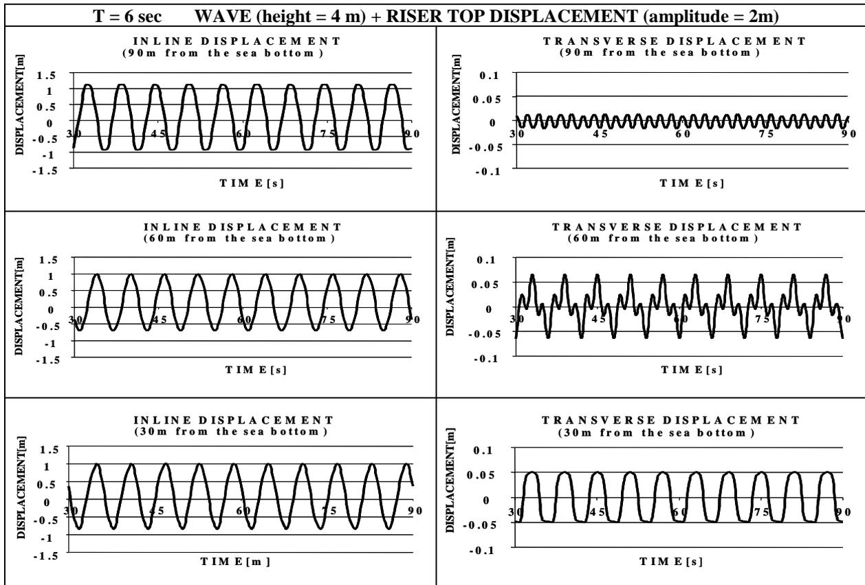
Figure 4. Riser inline and transverse displacements from simulations for three different locations along the riser for combined top displacement and wave excitations with 6 seconds wave period.
