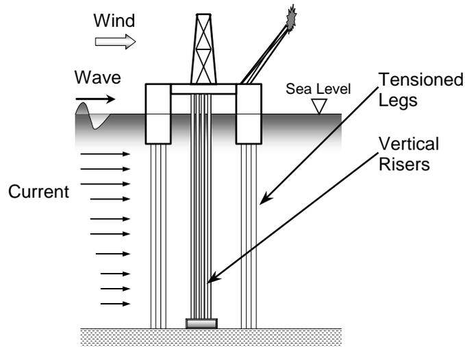
Figure 1. Typical configuration of riser and platform
