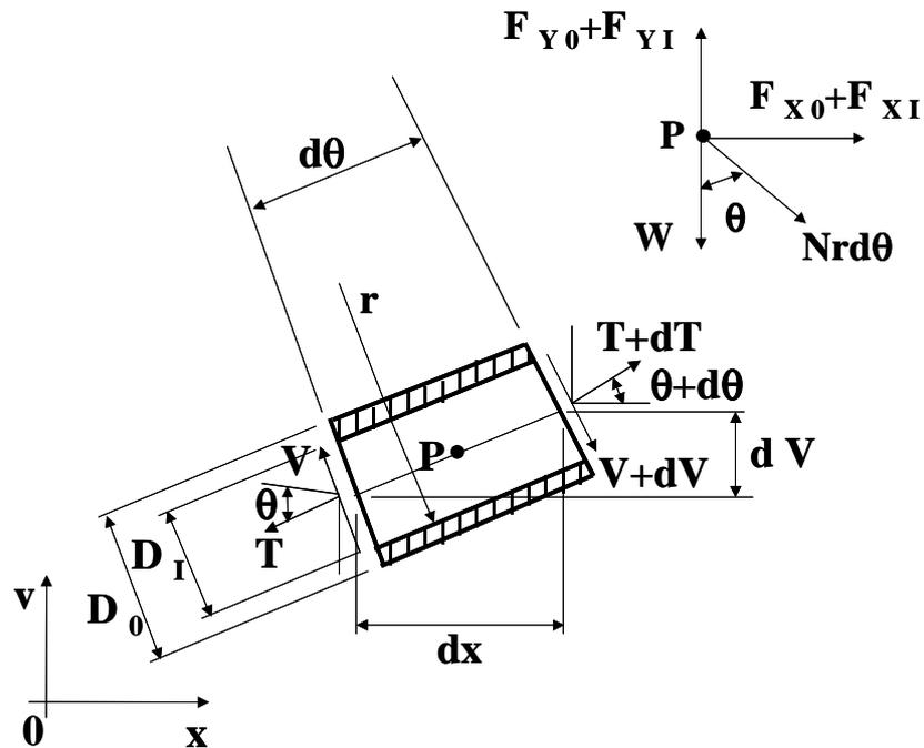
Figure 2. Scheme of equilibrium for a riser element
