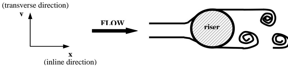
Figure 3. Scheme of a cross section of the riser and vortex formation
