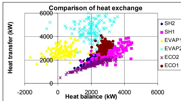
Figure 3 – Comparison between heat exchanged in different tube banks from heat balances and the rate of heat transfer considering zero heat transfer resistance.
