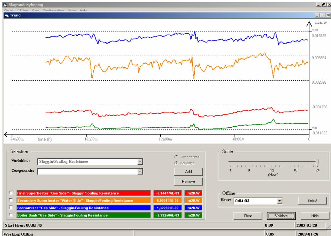
Figure 9 – Evolution of heat transfer resistance in Nyköping. (From the IST interface).
