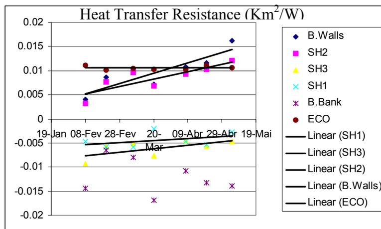
Figure 4 – Evolution of calculated heat transfer resistance along a heating period using gas temperatures.
