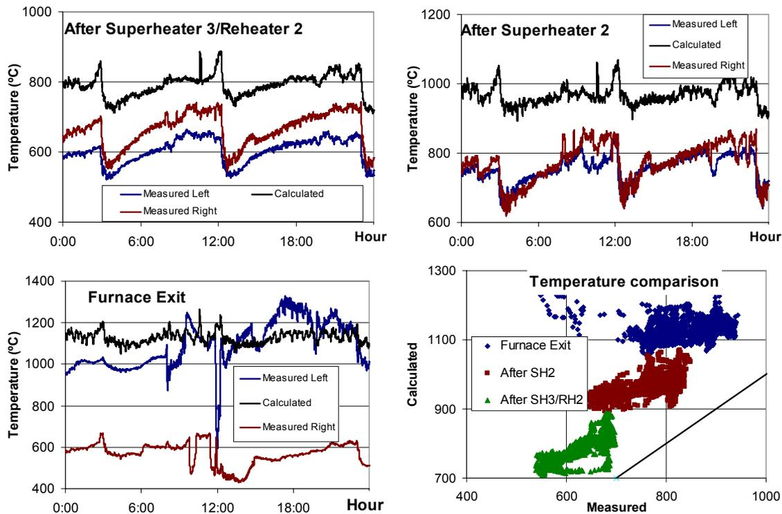
Figure 6 – Comparison between calculated and measured temperature in Upsalla a) Furnace exit, b) Above first tube panel, c) Above second tube panel, d) Comparison of calculated with average measured.
