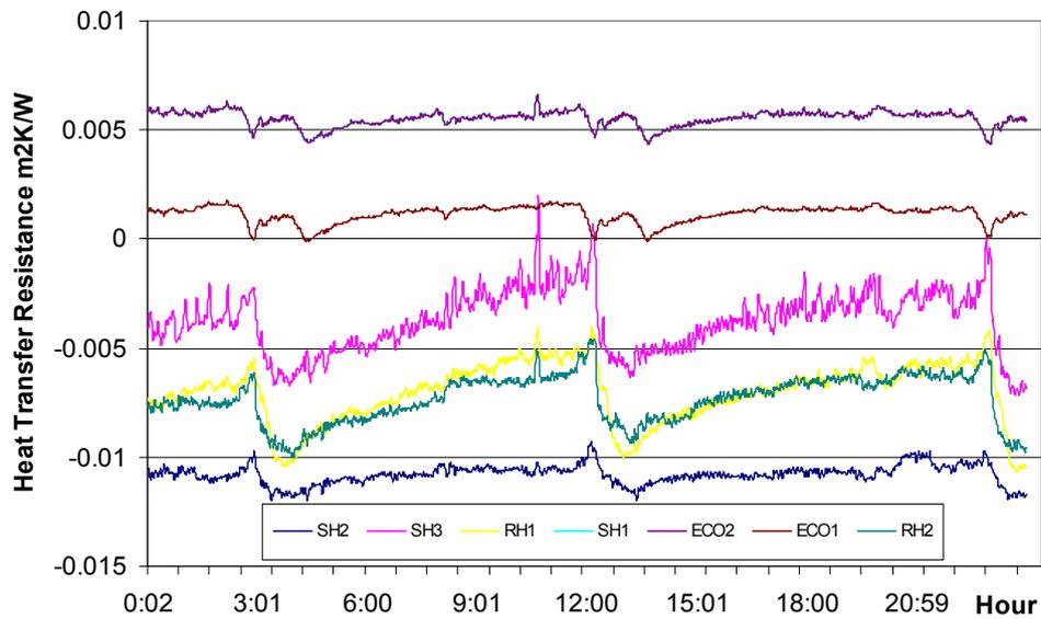
Figure 8 - Variation of heat transfer resistance during a day for Upsalla.
