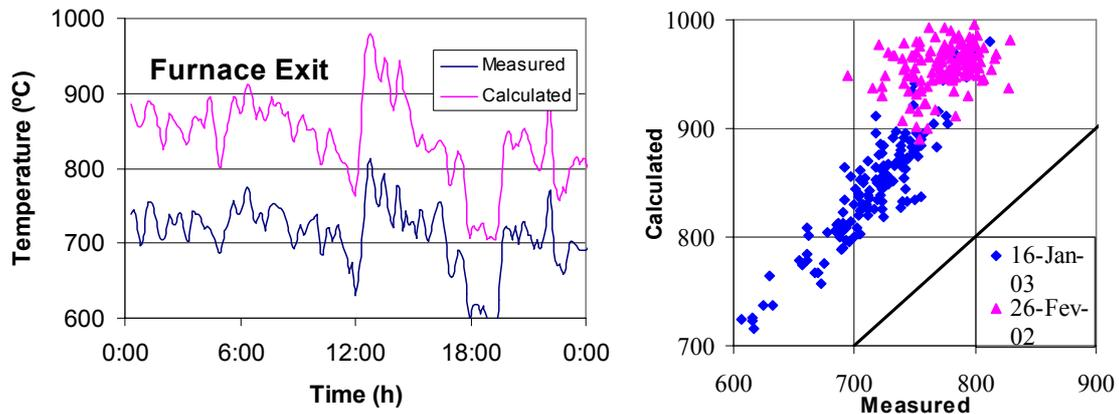
Figure 5 – Comparison between calculated and plant data furnace exit gas temperature in Mortágua boiler. a) Time evolution, b) Comparison for two different periods.
