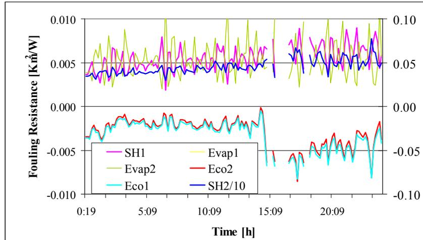
Figure 7 – Variation of heat transfer resistance during a day for Mortágua using olive stones (26/02/02).
