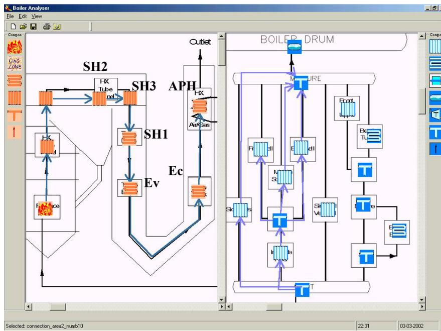
Figure 2 - Sketch of the gas circuit and water panels and tube banks for the evaporator in Nyköping.
