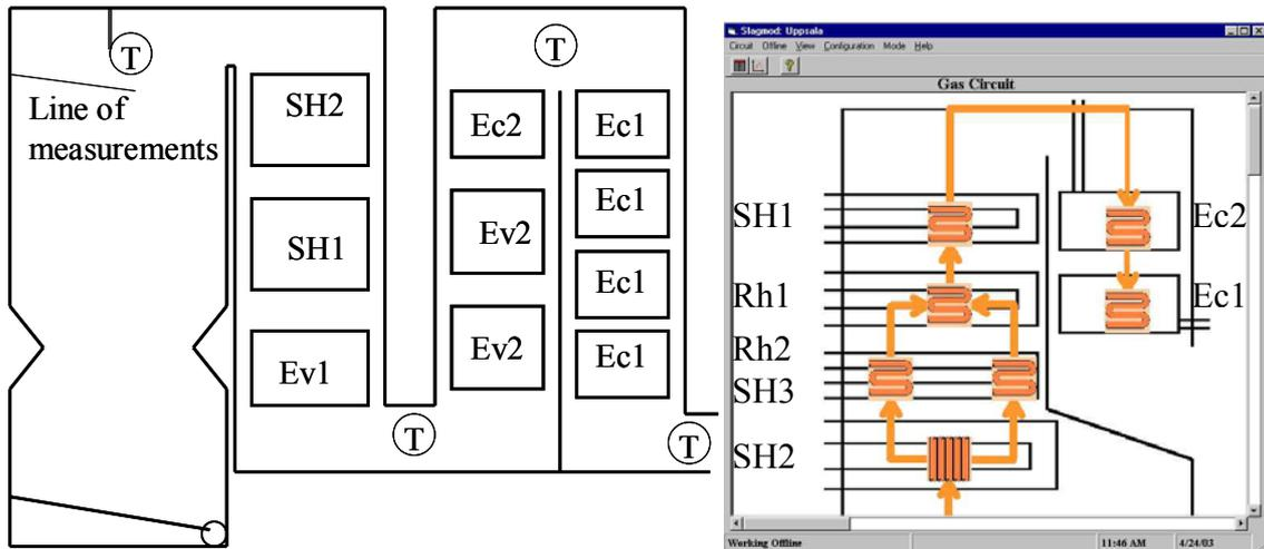
Figure 1 - Sketch of the gas circuits from plants. a) Mortágua (Indication is given of locations where temperature is measured), b) Upsalla (Sketch taken from the graphical interface installed at the plant).
