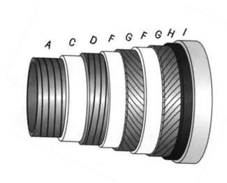
Figure 1. Typical Non - Bonded Flexible Riser
