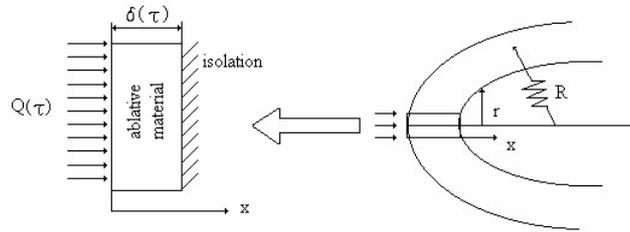
Figure 1. Schematic representation of ablative process in the stagnation point.
