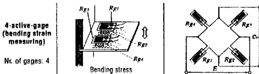
Figure 6. Arrangement of four strain gages forming a complete Wheatstone bridge.
