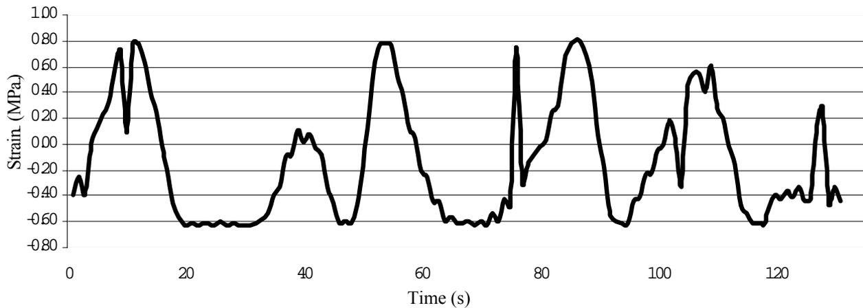
Figure 10. Behavior from the flexion strain due to him drags of pressure, in function of the time, for fluid velocity in the conduit of 0.170 m/s.
