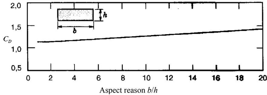
Figure 2.  $C_D$  as function of the aspect ratio,  $b/h$ , [Hoerner, 1965].
