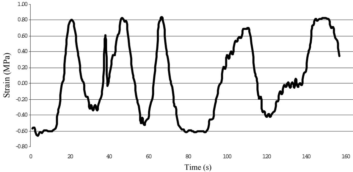
Figure 9. Behavior of the flexion strain due to the drag of pressure as function of the time, for fluid velocity in the channel of 0.07322 m/s.
