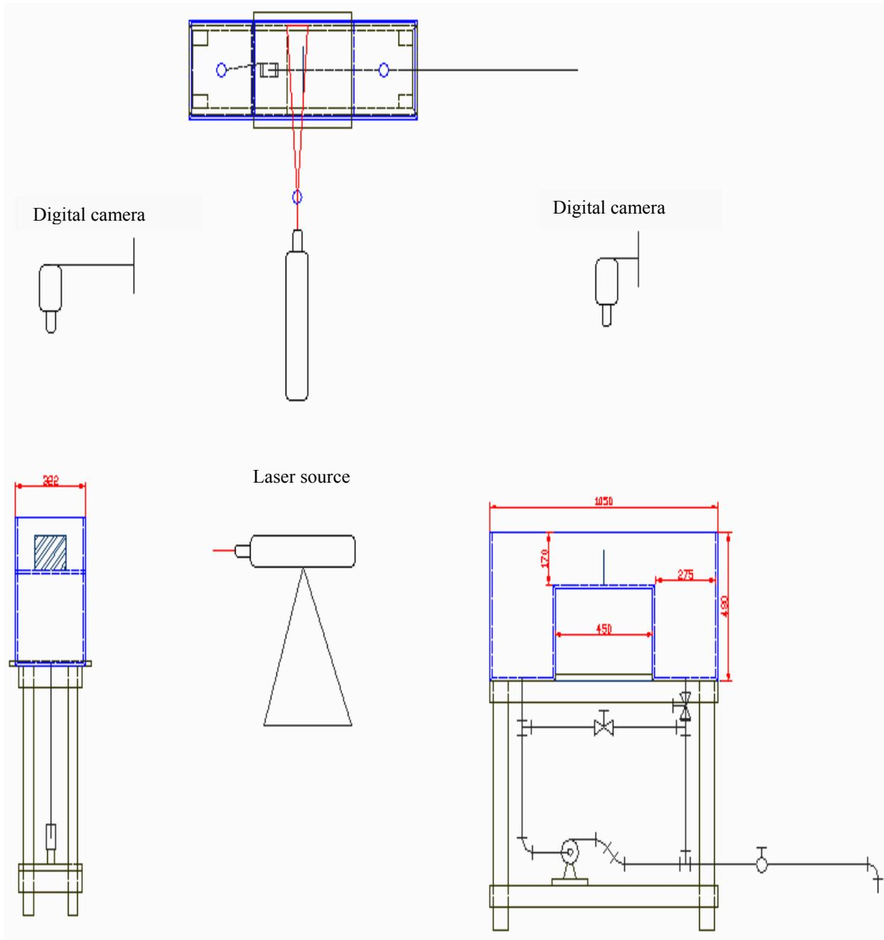
Figure 8. Assembly view for obtaining the velocity fields.
