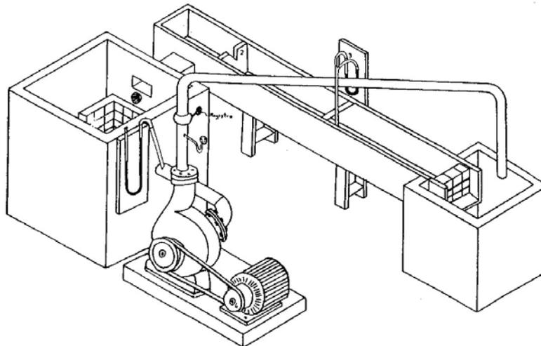
Figure 3. Rectangular channel used in the experiment.
