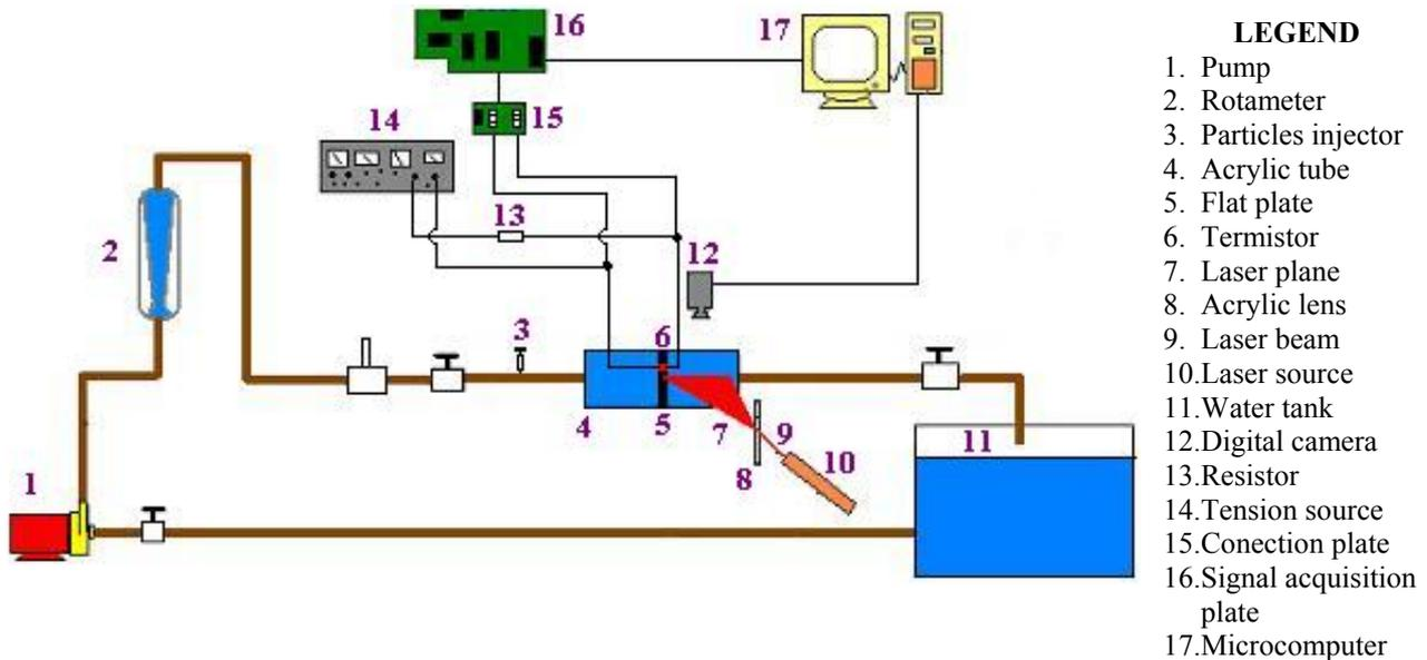
Figure 3. Tests Bench for study of vortex flow meter.
