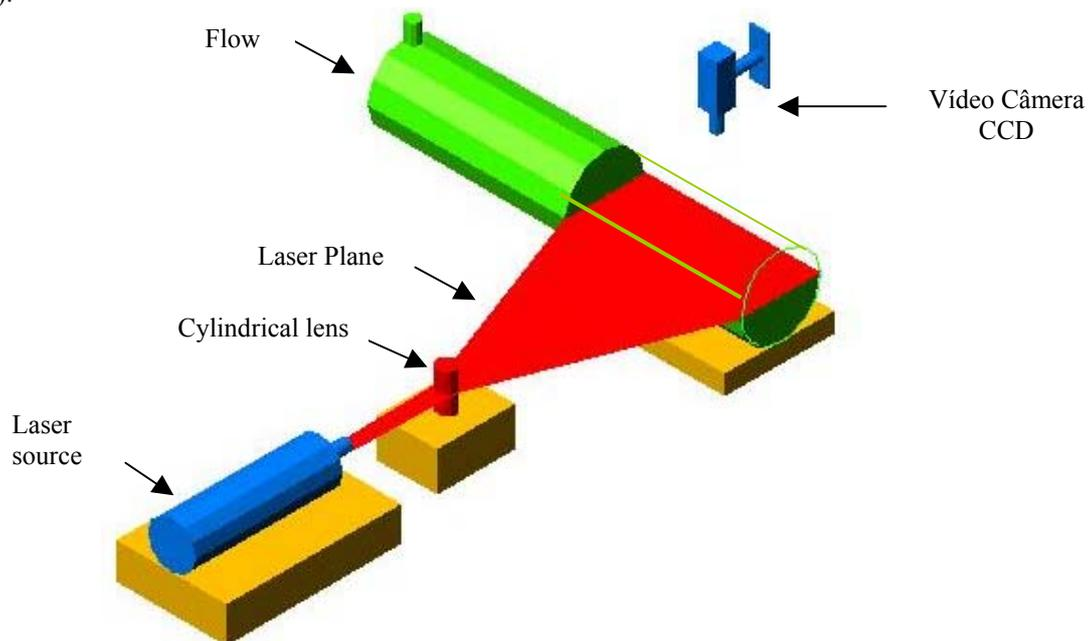
Figure 6. Three-dimensional scheme of the vortex visualization
