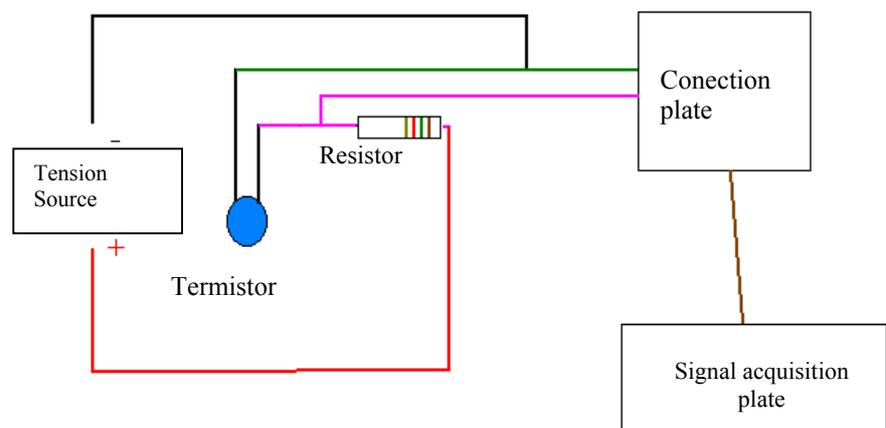
Figure 5. Scheme of sensor connection.
