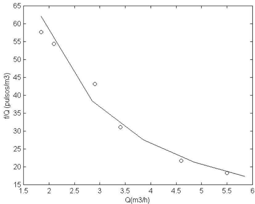
Figure 7. Calibration Curve of the vortex flow meter: factor of calibration  $f/Q$  (pulses/m<sup>3</sup>) x flow  $Q$  (m<sup>3</sup>/h)
