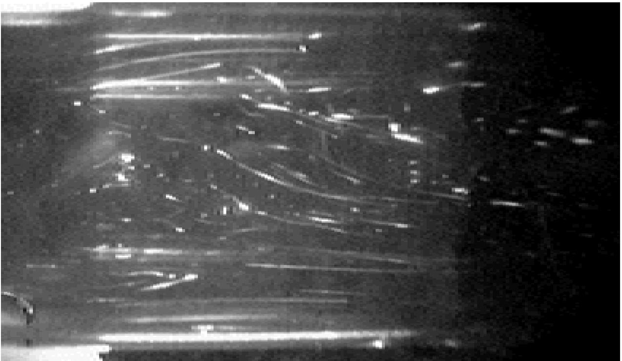
Figure 9. Image of vortex for flow of  $5.0 \text{ m}^3/\text{h}$  ( $t=0.166\text{s}$ ).
