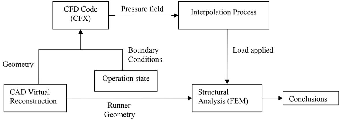
Figure 1. Uncoupled fluid-structure interaction project sequence.
