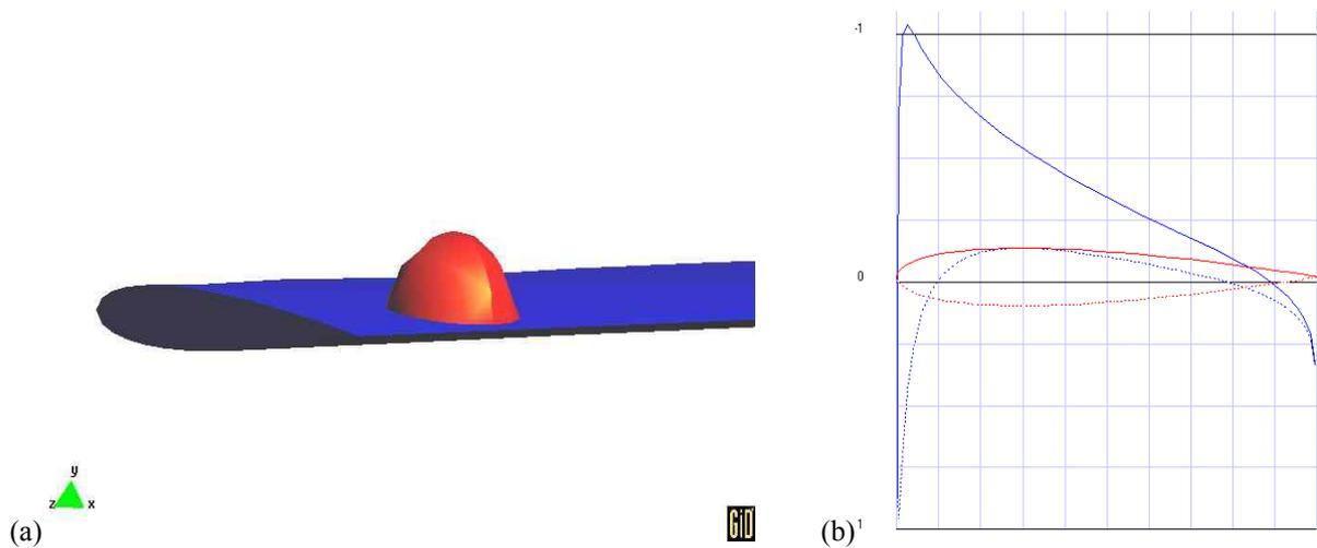
Figure 3. Semi-sphere interpolation domain over airfoil (a) and  $C_p$  distribution for this airfoil (b).
