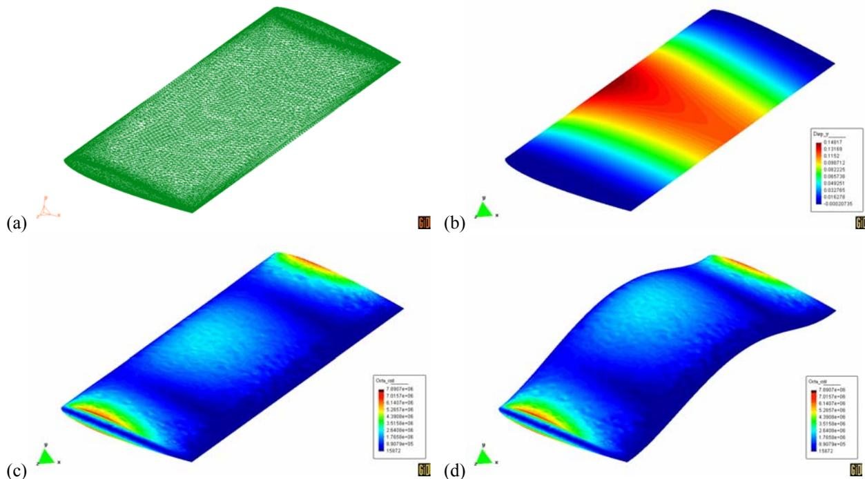
Figure 7. Mesh used, displacements and critical stresses over the airfoil.
