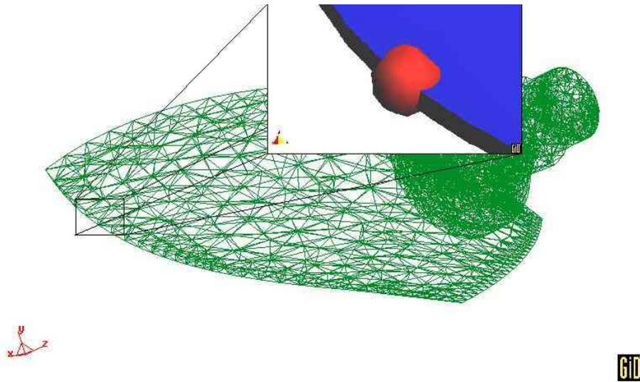
Figure 2. Sphere interpolation domain crossing thin trubine blade.
