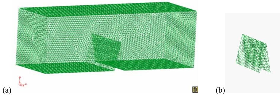
Figure 4. Solid mesh representing flow problem and surface mesh representing structural boundary conditions.
