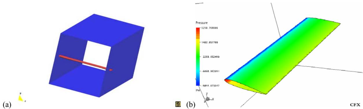
Figure 6. Geometry and pressure distribution over airfoil.
