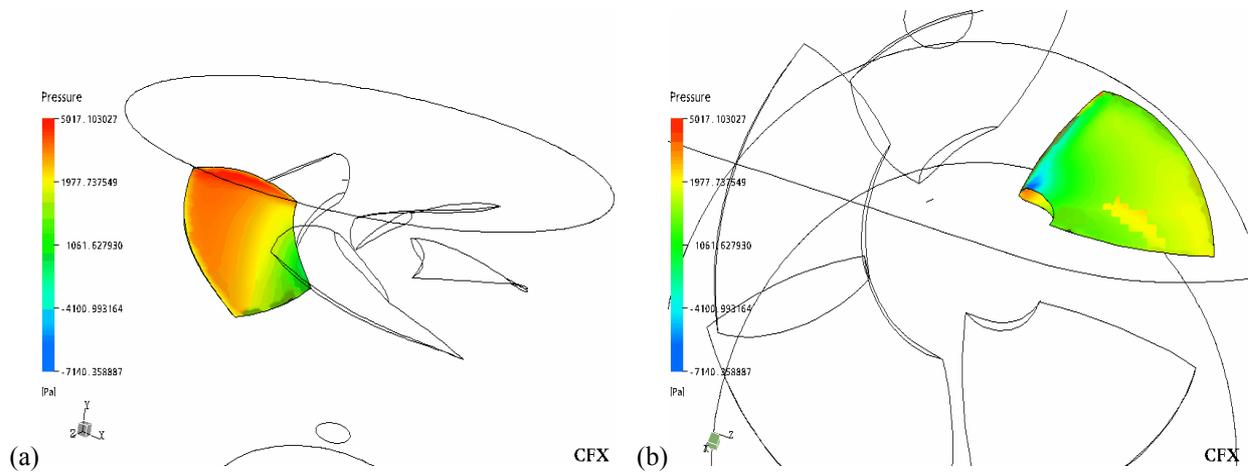
Figure 8. Simulated pressure distribution for a turbine blade.
