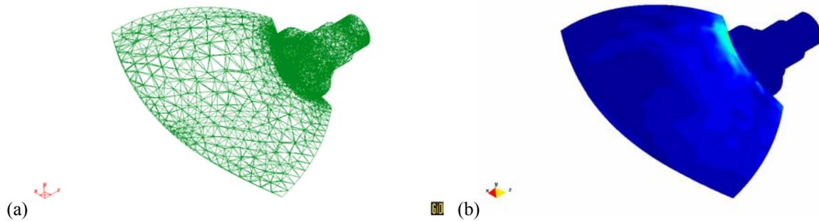
Figure 9. Solid mesh and critical stresses for the blade simulation.
