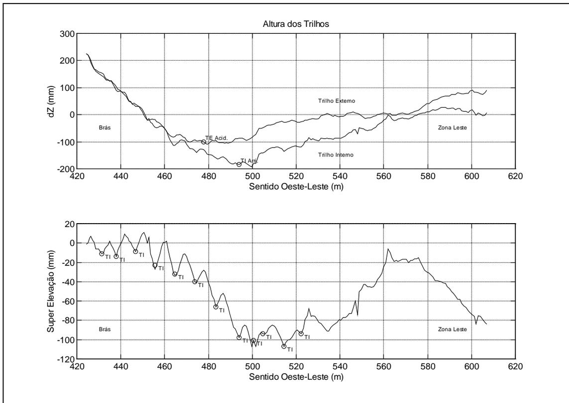
Figure 5 a) Track height and b) super-elevation
