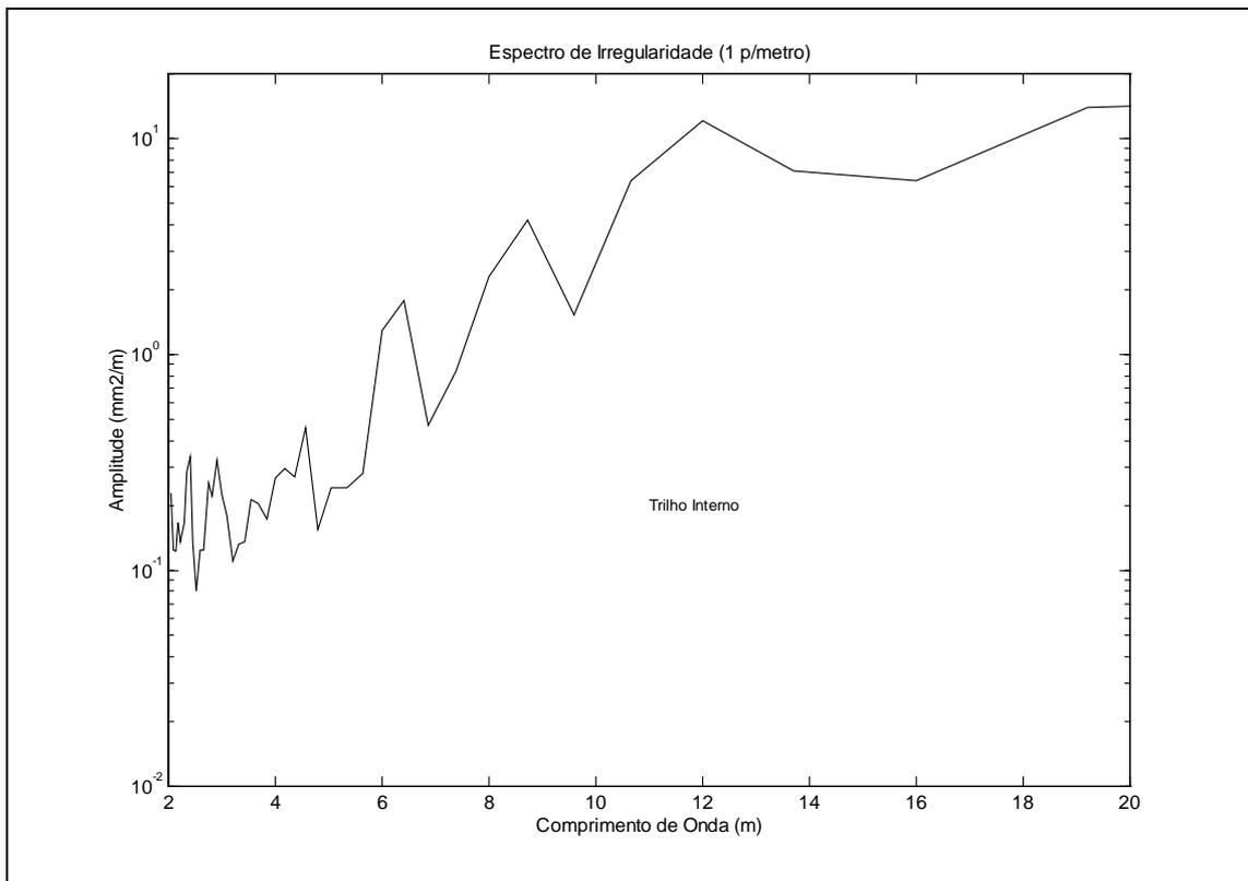
**Figure 8 – Vertical Track Wavelength Analysis**
