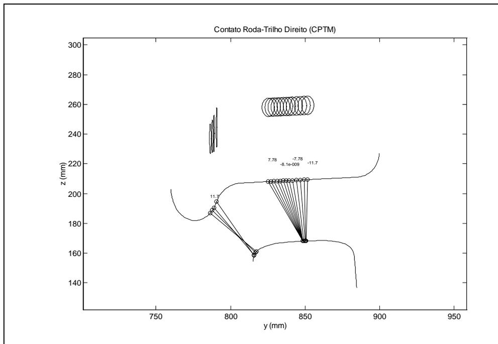
Figure 3 – Contact point and ellipse size between wheel/rail
