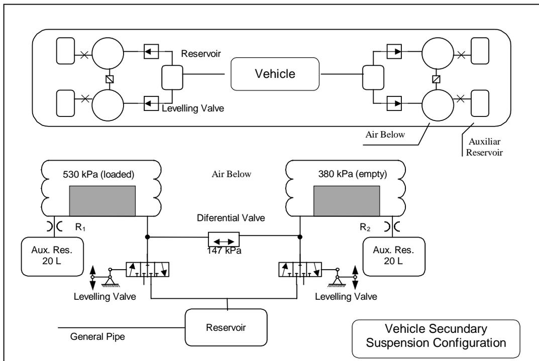
**Figure 2 – Pneumatic Secondary Suspension**
