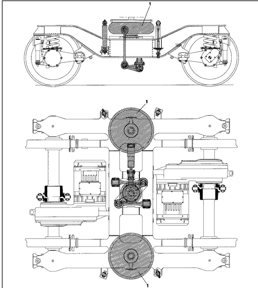
**Figure 1 – Truck suspension details**
