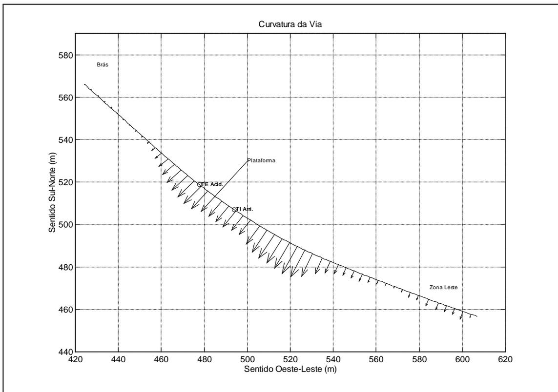
Figure 6 – Track Curvature (arrow size represents curvature magnitude)
