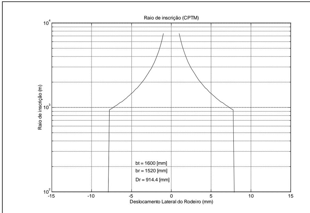
Figure 4 – Pure rolling curve radius
