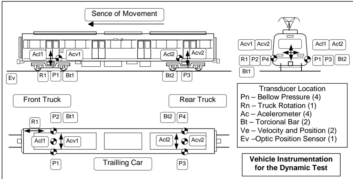
Figure 9 – Transducer locations for on track dynamic measurements
