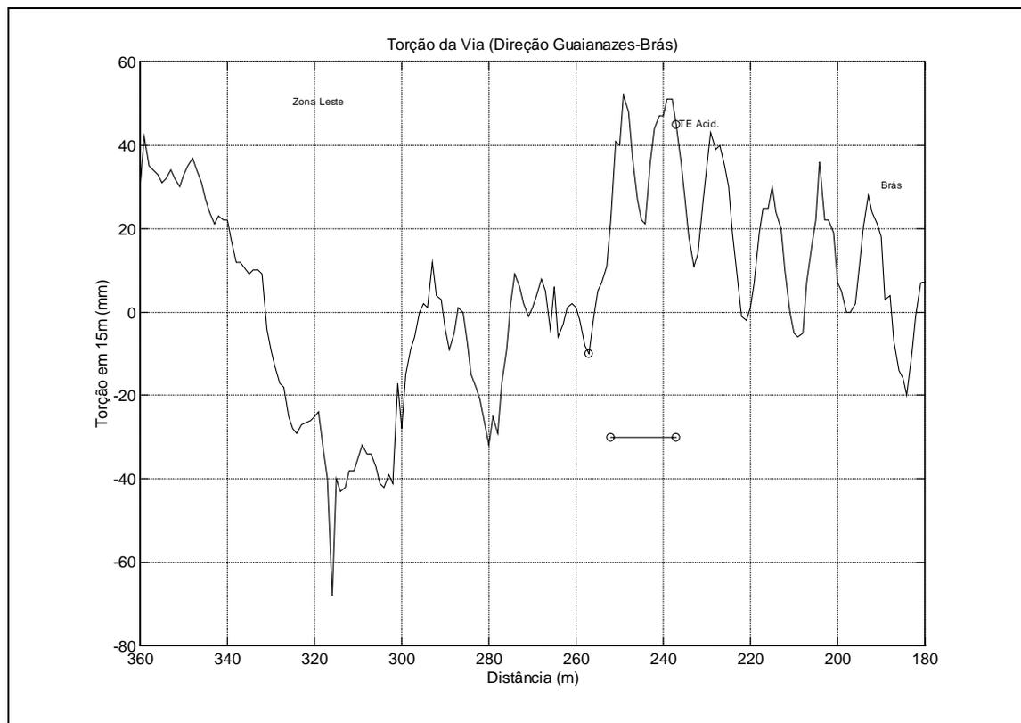
**Figure 11 - Track twist (over vehicle length basis)**
