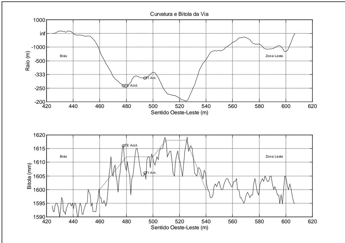
**Figure 7a Track curvature b) track gage**
