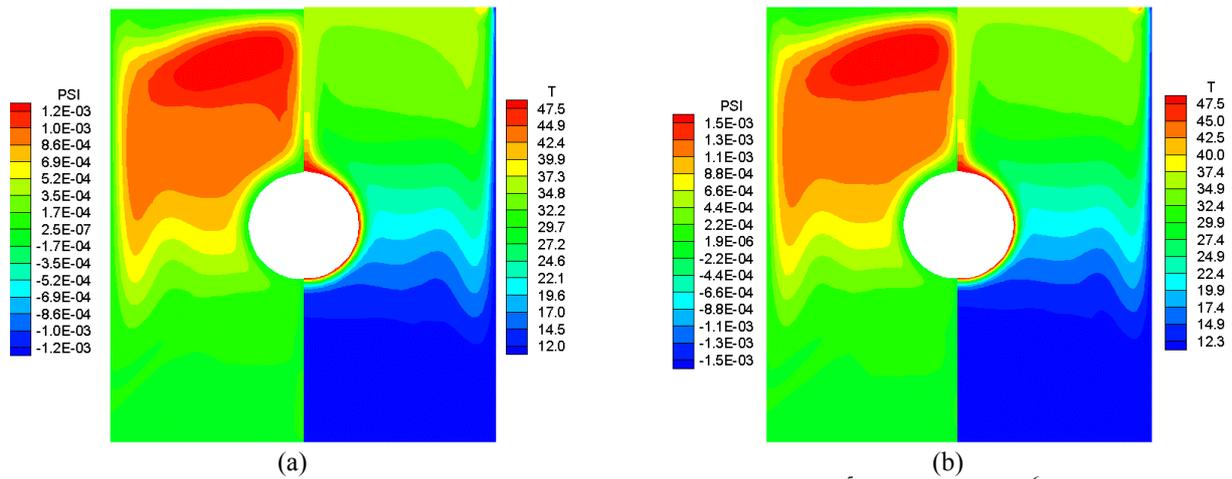
Figure 8. Streamfunction PSI and Temperature T[°C] for W=3,6 (a)  $Ra = 5,5 \times 10^5$  (b)  $Ra = 1,0 \times 10^6$
