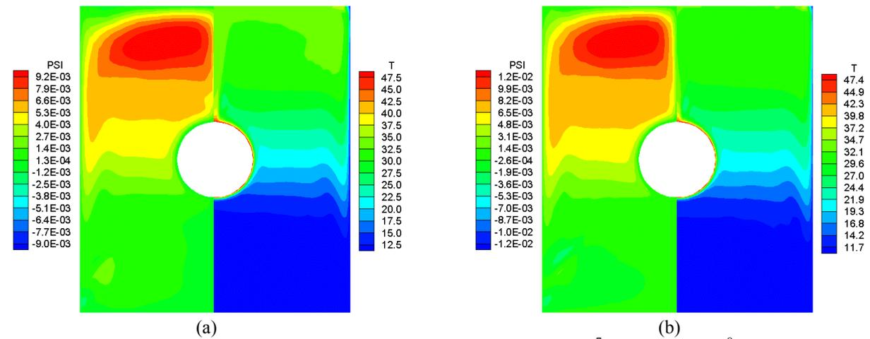
Figure 10. Streamfunction PSI and temperature T[°C] for W=3,6 (a)  $Ra = 5,5 \times 10^7$  (b)  $Ra = 1,0 \times 10^8$
