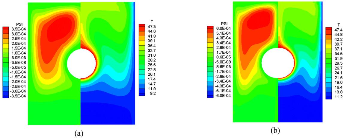
Figure 5. Streamfunction PSI and Temperature T[°C] for W=2,9. (a)  $Ra = 1,0 \times 10^4$  (b)  $Ra = 7,5 \times 10^4$
