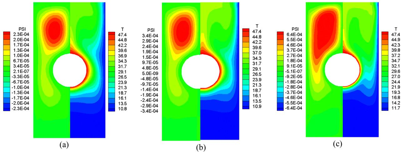
Figure 4. Streamfunction PSI and Temperature T[°C] for W=2,1. (a)  $Ra = 1,3 \times 10^3$  (b)  $Ra = 5,0 \times 10^3$  (c)  $Ra = 7,5 \times 10^4$ .
