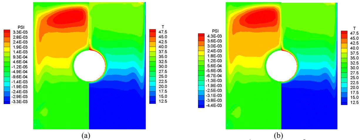
Figure 9. Streamfunction PSI and Temperature T[°C] for W=3,6 (a)  $Ra = 5,5 \times 10^6$  (b)  $Ra = 1,0 \times 10^7$
