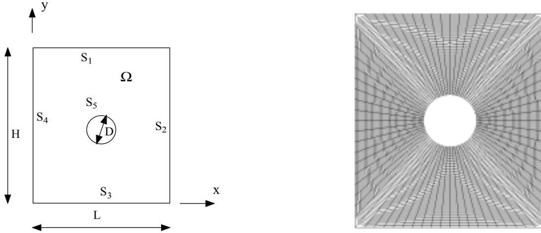
Figure 1. Geometry and typical grid of the present work
