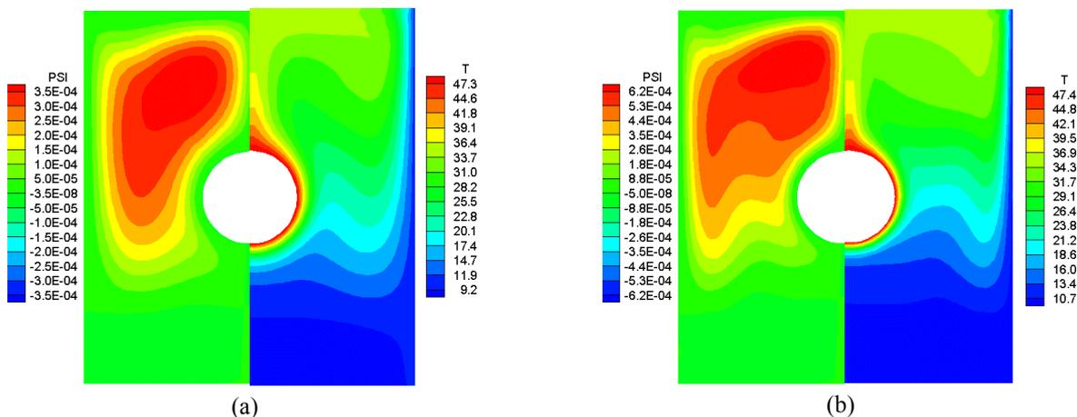
Figure 6. Streamfunction PSI and Temperature T[°C] para W=3,6 (a)  $Ra = 1,0 \times 10^4$  (b)  $Ra = 7,5 \times 10^4$
