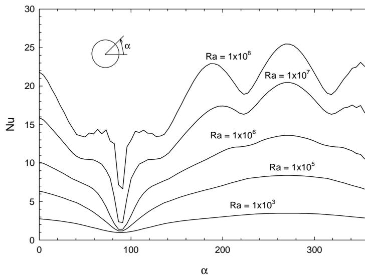
Figure 7. Local Nusselt number  $Nu$  versus angle  $\alpha$  for  $Ra = 1,0 \times 10^3$  to  $1,0 \times 10^8$  and aspect ratio  $W=3,6$
