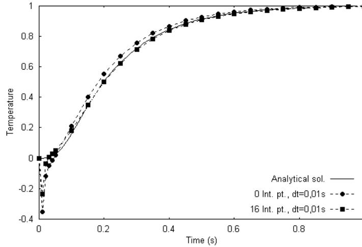
Figure 4. The poles effect in a mesh with 26 nodes when the time step is equal 0,01s.
