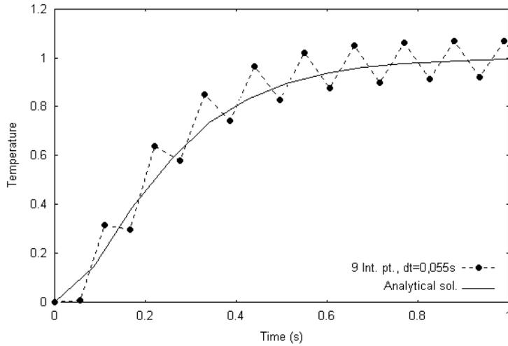
Figure 6. Mesh with 64 nodes, 9 poles and time step equal 0,055s.
