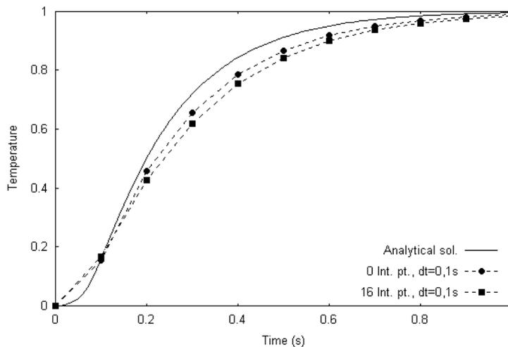
Figure 3. The poles effect in a mesh with 26 nodes when the time step is equal 0,1s.
