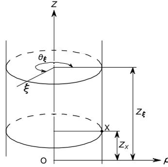
Figure 1. Cylindrical coordinates for an axisymmetric body.
