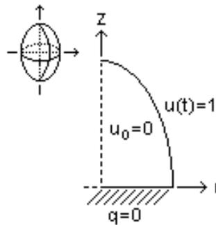
Figure 5. Geometric model for prolate spheroidal solid.
