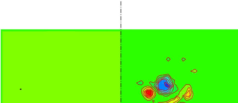
(g) vortex cloud with turbulence modeling (t=30): point (6) in the Fig. (2)
