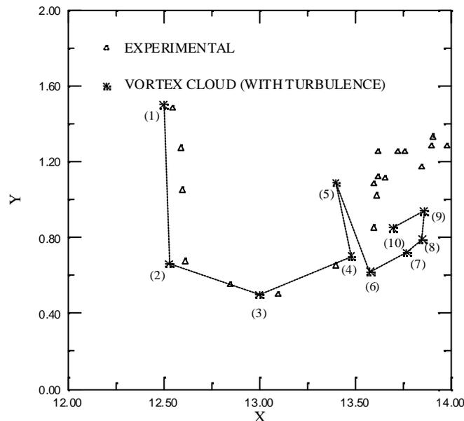
Figure 2. Trajectory of the free vorticity from wing tips
