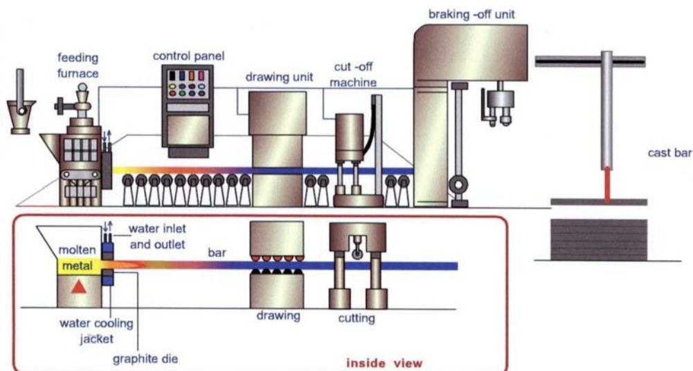
Figure 1. Continuous casting of cast iron bars.
