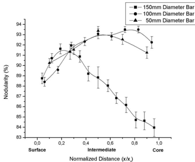
Figure 8. Nodularity as a function of the normalized distance in the continuous casting bars.
