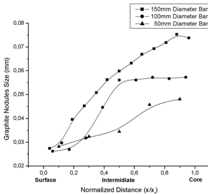
Figure 5. Graphite nodules size as function of the normalized distance in the continuous casting bars.
