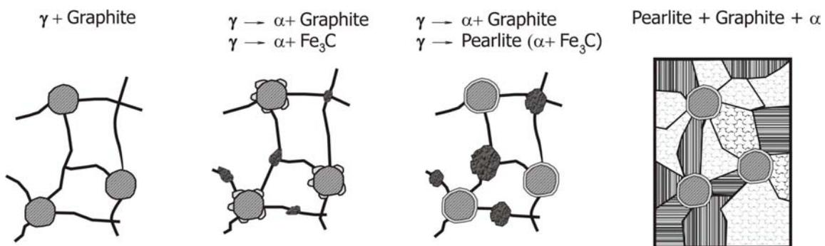
Figure 2. Eutectoid transformations sequence in ductile iron, according to Johnson & Kovacs (1978).
