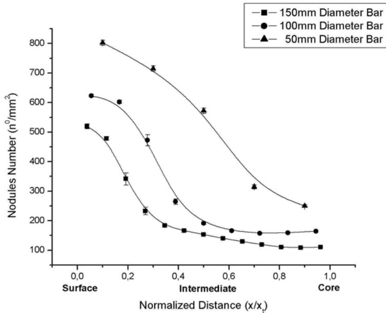
Figure 4. Graphite nodules number as function the normalized distance in the continuous casting bars.
