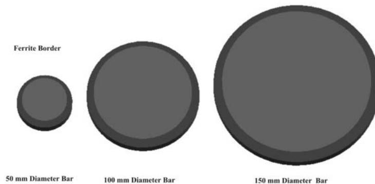
Figure 7. Ferritic rim of the continuous casting bars.
