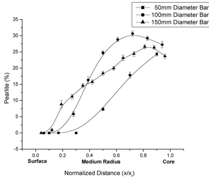
Figure 6. Amount of Pearlite as a function of the normalized distance in the continuous casting bars.
