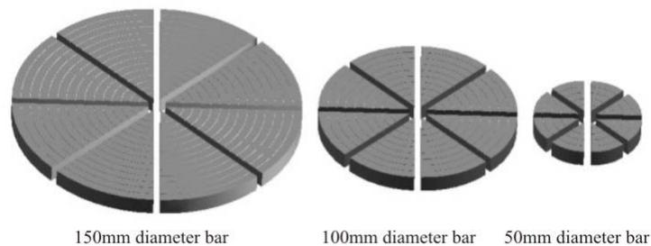
Figure 3. Continuous casting bars showing fashion that the samples were analyzed.
