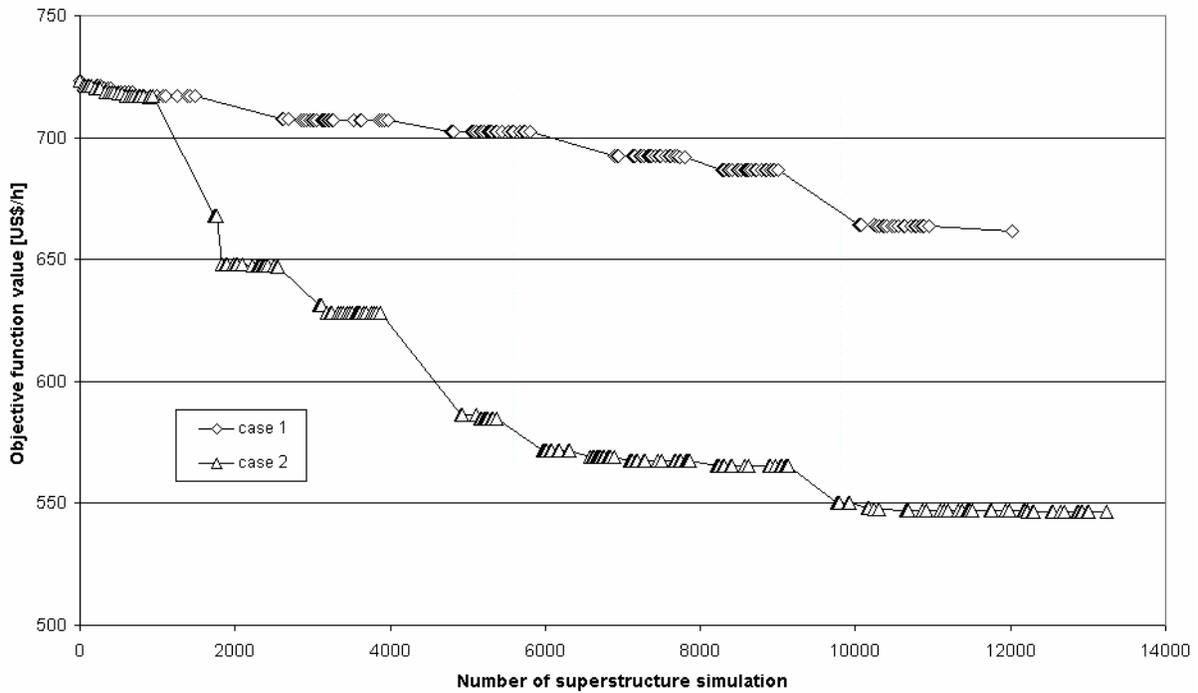
Figure 5. Objective function variation for Cases 1 and 2 throughout the optimization process of the superstructure shown in Fig. (2).
