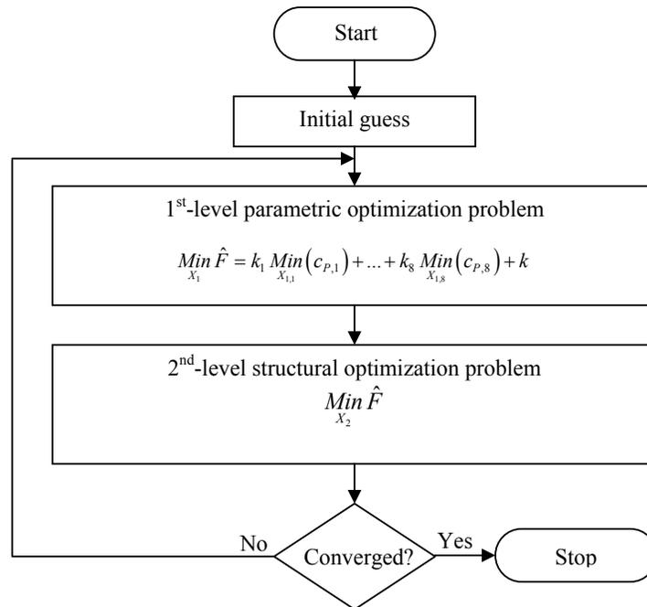
Figure 3. Iterative process for the multilevel optimization problem.
