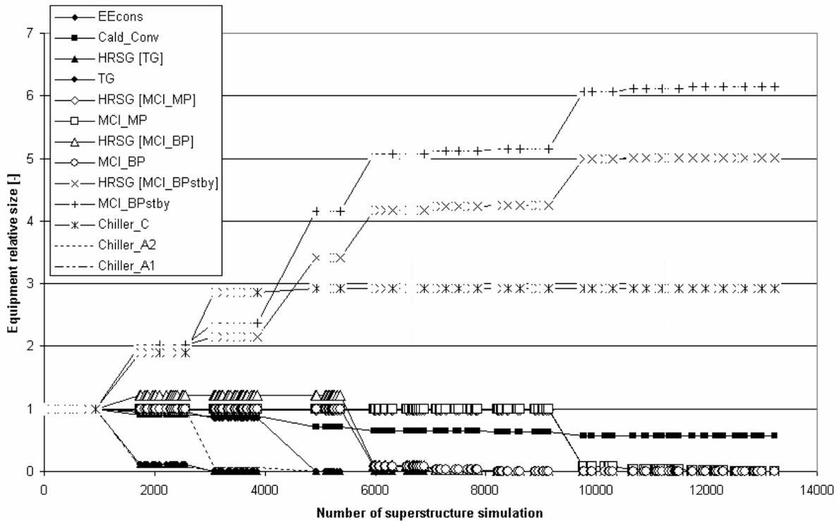
Figure 6. Evolution of the configuration of the cogeneration system for Case 2 throughout the optimization process of the superstructure shown in Fig. (2).
