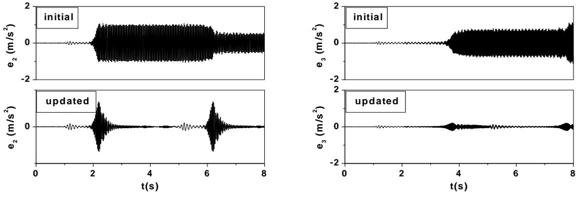
Figure 5: Residue of the second and third accelerometers.
