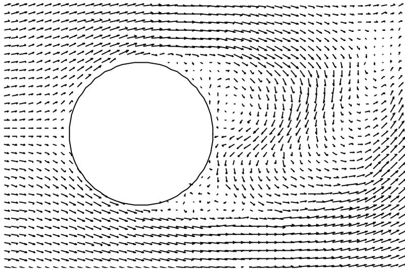
Figure 2. Instantaneous velocity field at  $t=40$  around a circular cylinder.
