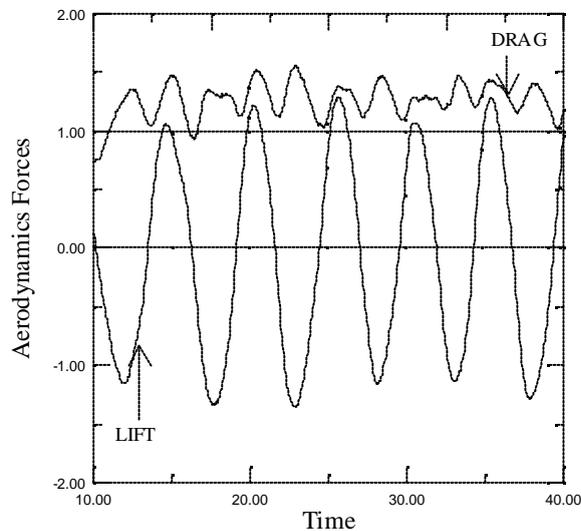
Figure 3. Time history of the aerodynamics loads at Reynolds number  $\text{Re}=10^4$ .
