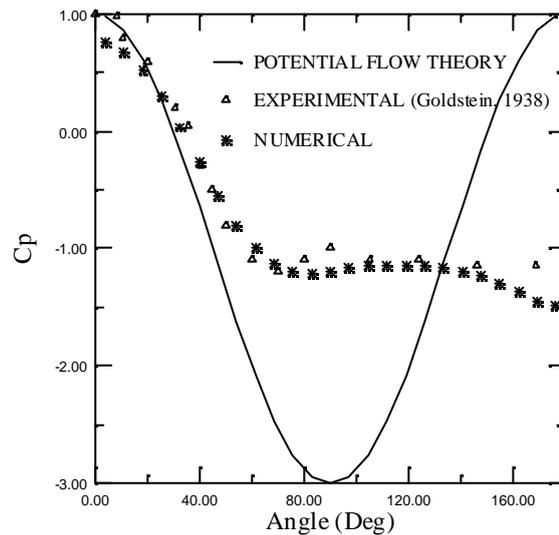
Figure 4. Predicted pressure distribution for circular cylinder at Reynolds number  $Re=10^4$ .
