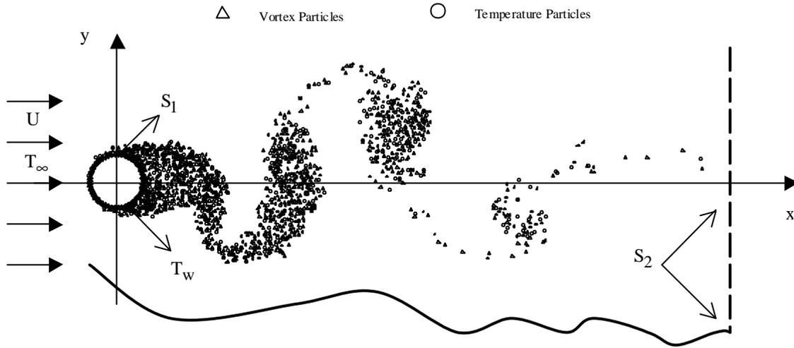
Figure 1. Flow around a bluff body.
