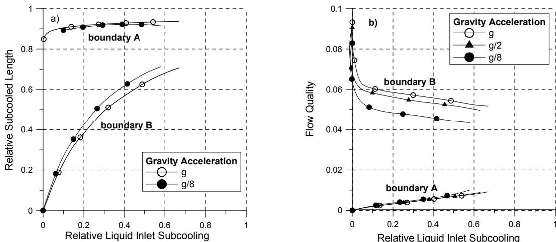
Figure 7. a) Subcooled length and b) Flow quality along both boundaries for different values of gravity acceleration.
