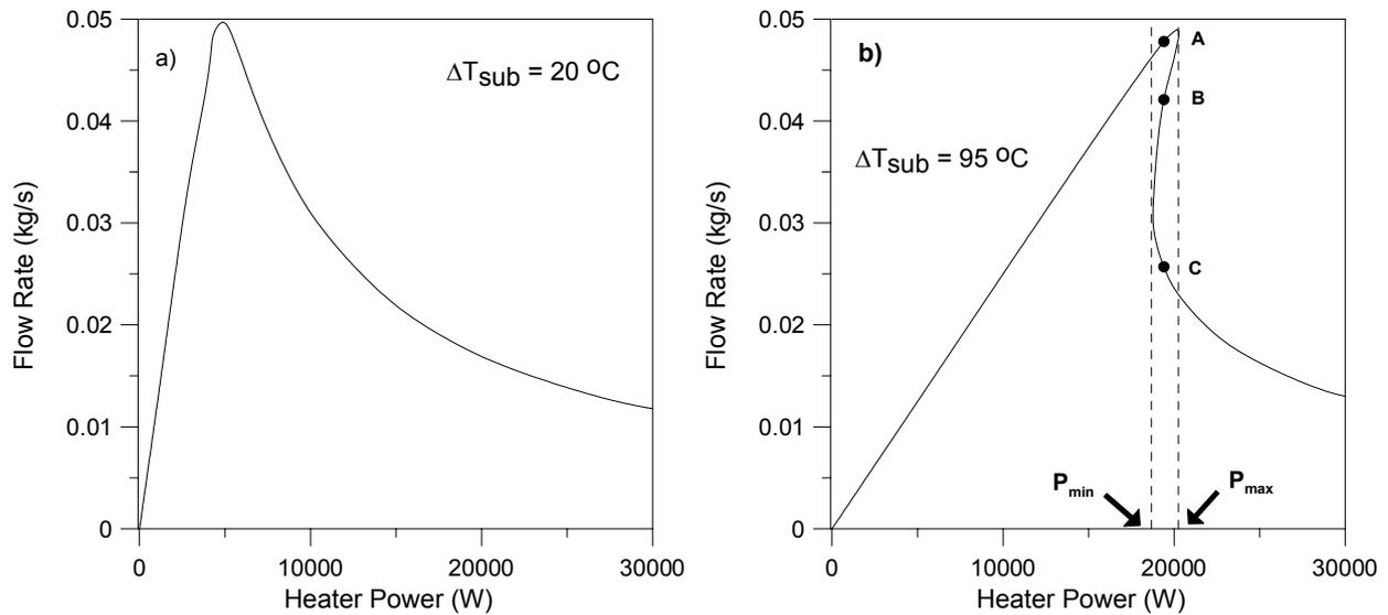
Figure 2. Natural circulation flow rate as function of heater power for different liquid inlet subcoolings using the loop parameters in Table 1.
