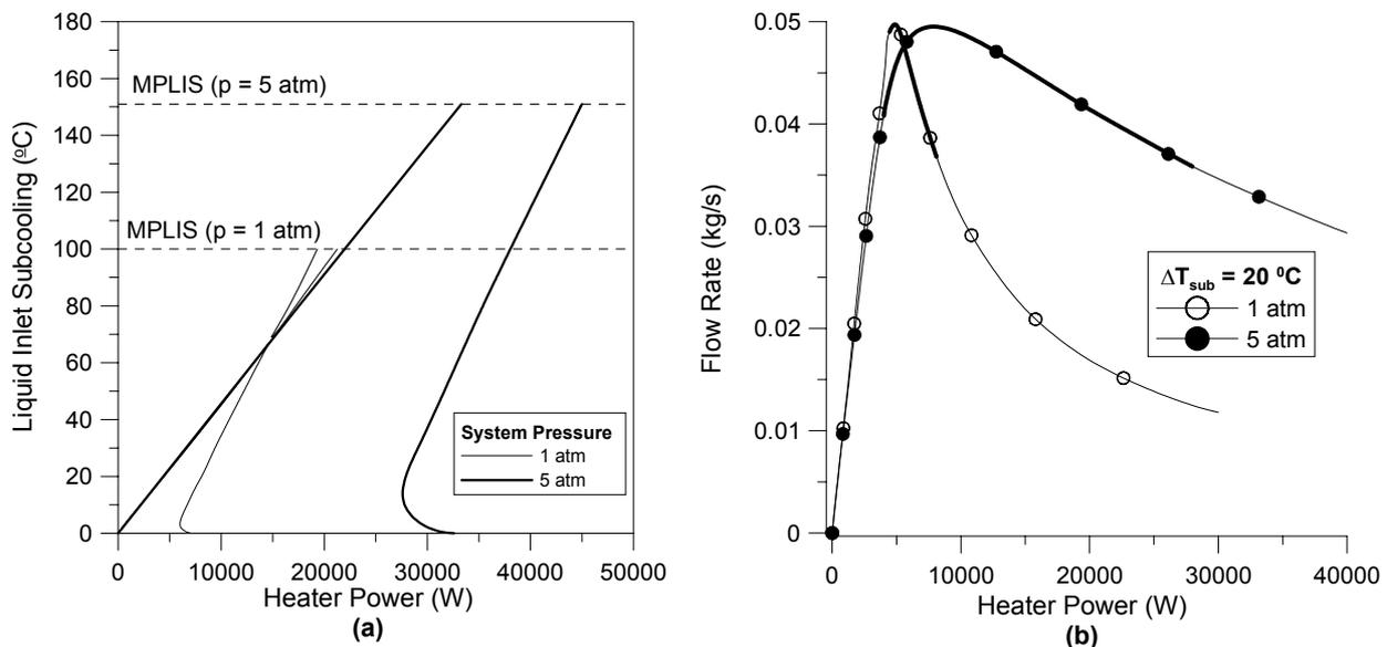
Figure 8. a) Stability maps; and b) Naturally induced loop flow rates as function of heater power for different values of system pressure. The thicker portions of the curves refer to the stable system operating points.
