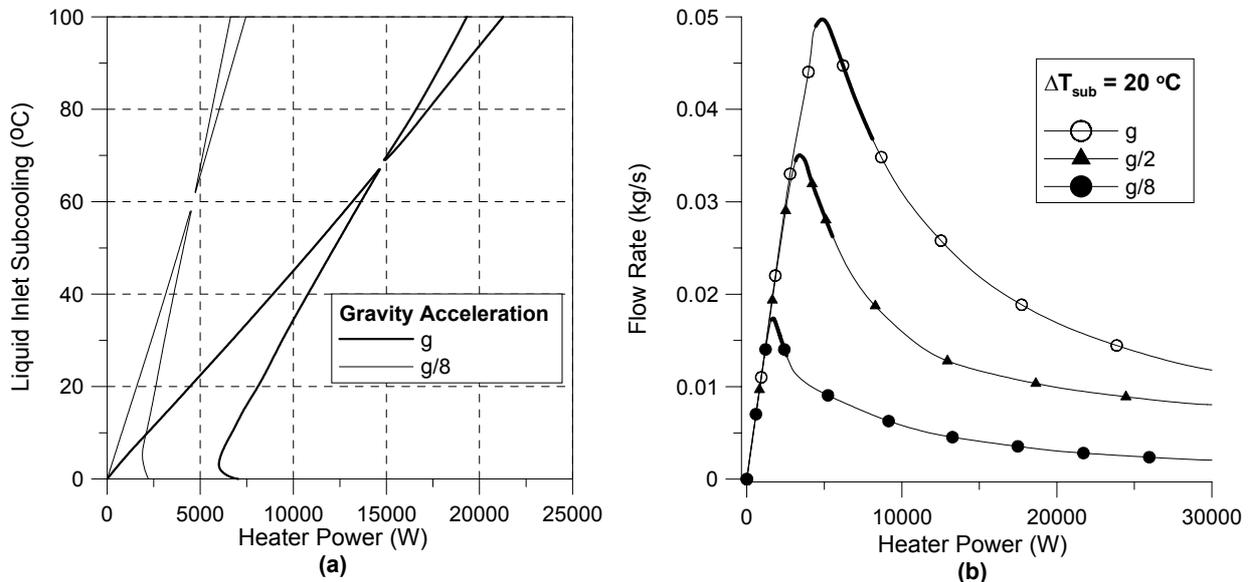
Figure 6. a) Stability maps; and b) Naturally induced loop flow rate as function of heater power for different values of gravity acceleration.
