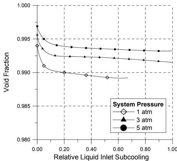
Figure 10. Void fraction variation along boundary B for different system pressure.
