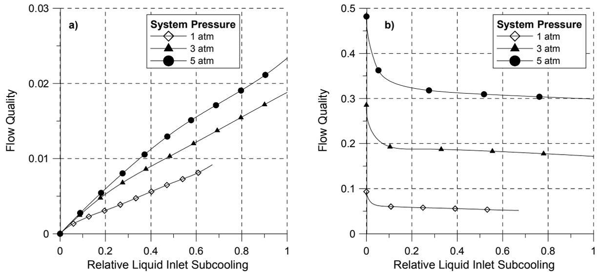
Figure 9. Flow quality at (a) boundary A and (b) boundary B, for different values of system pressure.
