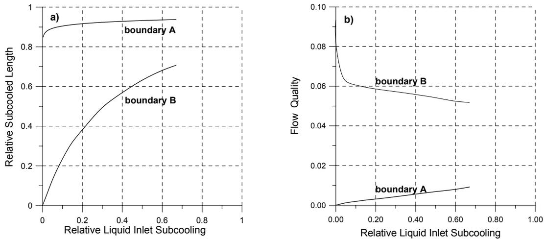
Figure 4. a) Relative Subcooled length  $[\lambda/(d - c)]$  and b) Flow quality along both boundaries shown in Fig. 3 as function of the relative liquid inlet subcooling  $[\Delta T_{sub}/T_{sat}]$ .
