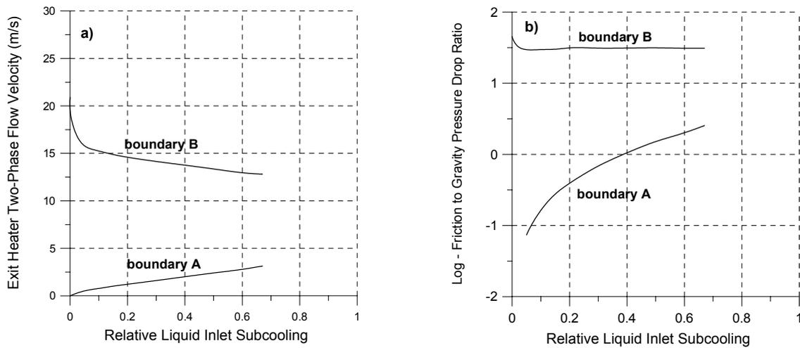
Figure 5. a) Two-phase flow velocity at the heater exit, and b) Ratio of the frictional to gravitational pressure losses in the two-phase part of the loop along both boundaries.
