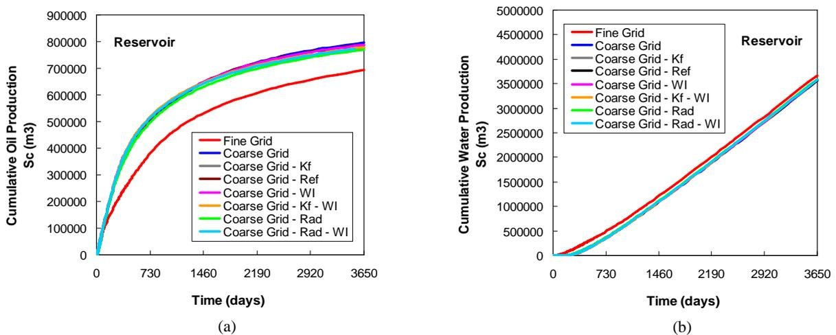
Figure 4. Presence of channels – (a) Reservoir cumulative oil production
