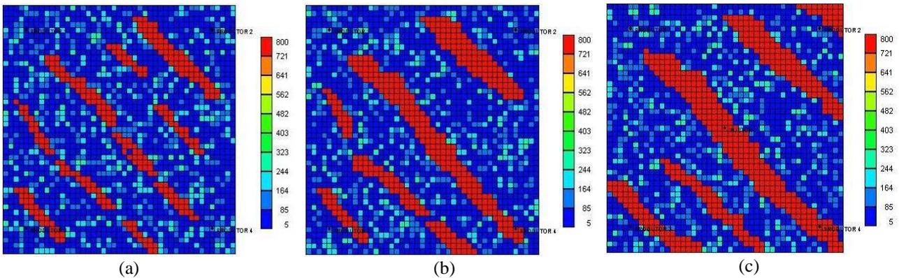
Figure 1. Fine grid with channels - Permeability distribution in x direction for: (a) Layer 1, (b) Layer 2 and (c) Layer 3.
