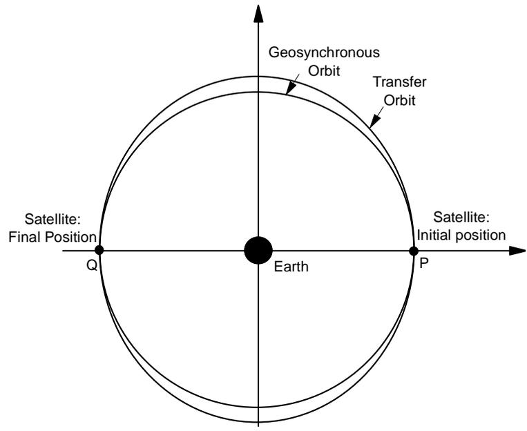
Figure 5. Orbit Transfer for a Geosynchronous Satellite.
