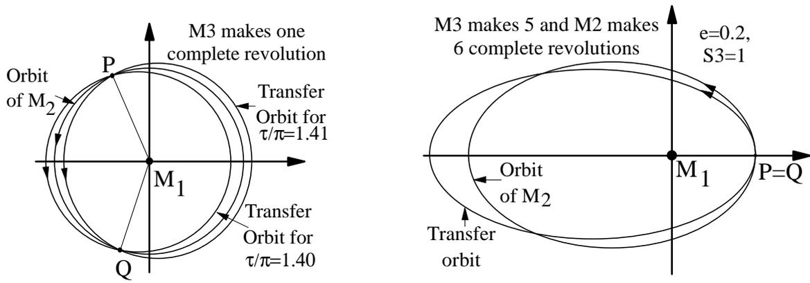
Figure 4. Some Transfer Orbits with Small  $\Delta V$ .
