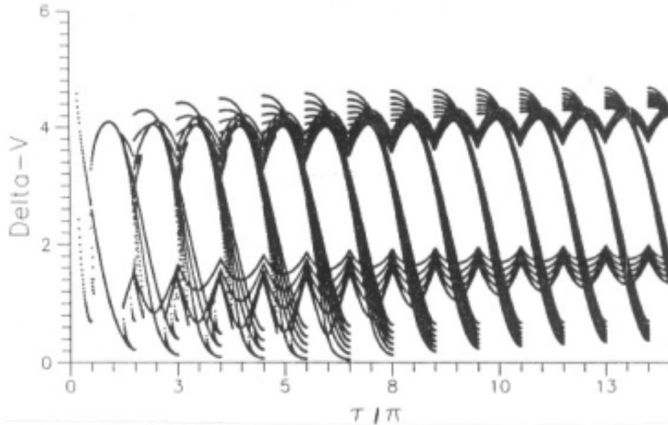
Figure 6. ( $\Delta V$ )vs( $\tau/\pi$ ) to Transfer a Geosynchronous Satellite (Elliptic Transfer Orbits).
