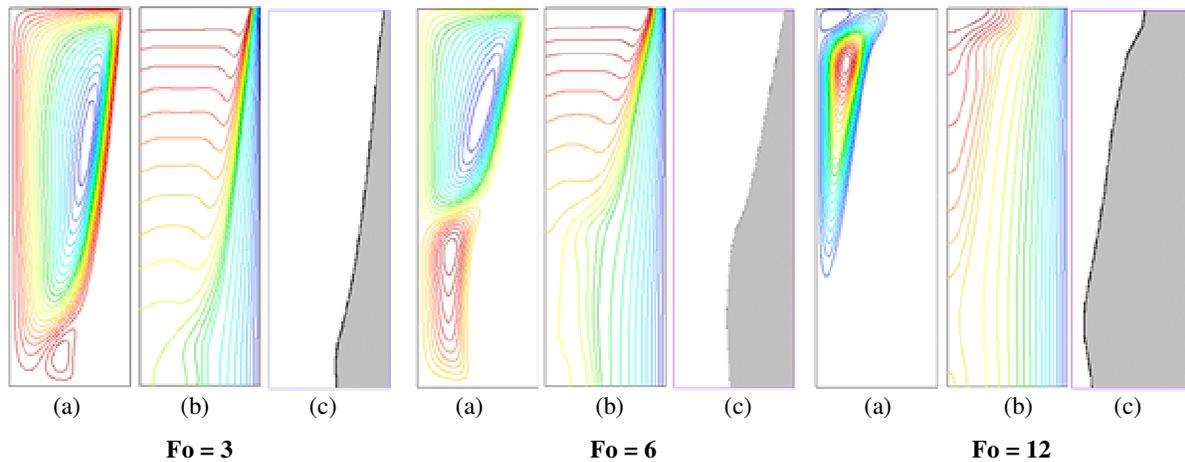
**Figure 4.** Intermediate numerical results: (a) streamlines; (b) isotherms and (c) formed ice.
