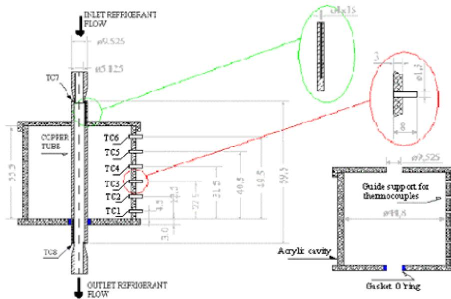
**Figure 1.** Test section.
