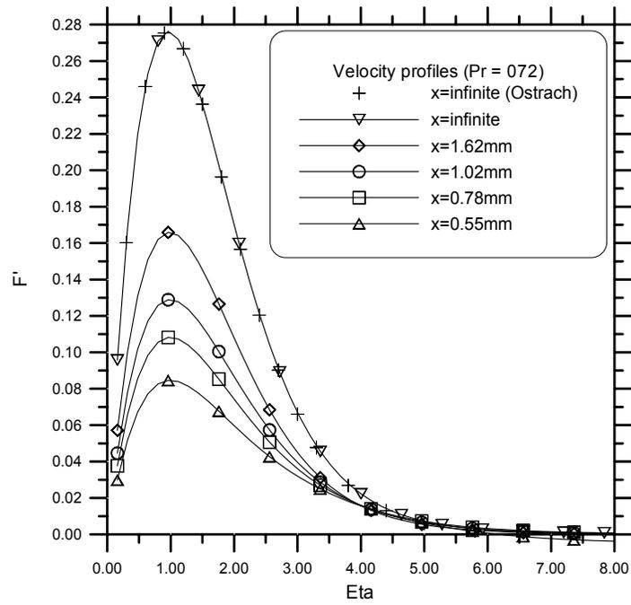
Figure 2. Velocity profiles for various distances form de leading edge
