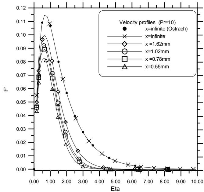
Figure 4. Velocity profiles for various distances from the leading edge locations Pr = 10
