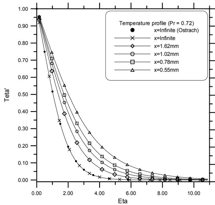
Figure 3. Temperature profiles for various distances form de leading edge Pr = 0.72
