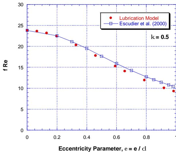
Figure 3:  $f \times Re$  as a function of eccentricity parameter predicted by the lubrication model is complete two-dimensional solution.
