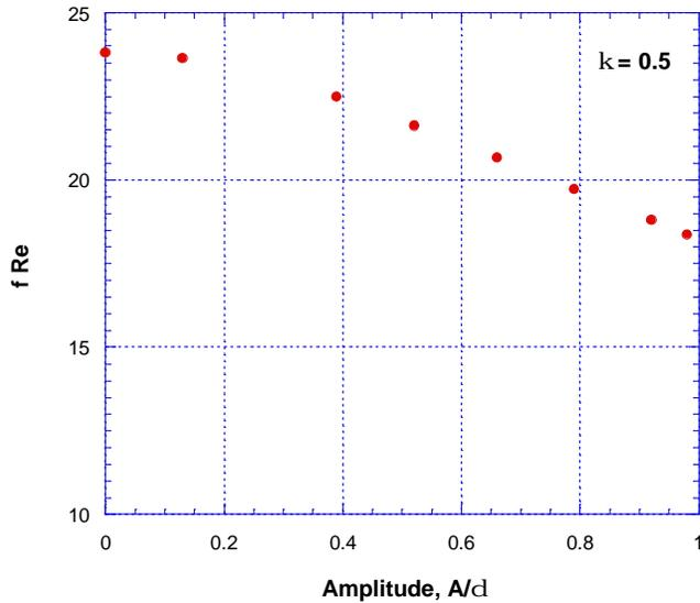
Figure 11: Friction factor as a function of the amplitude of the sinusoidal variation of the eccentricity along the main flow direction.
