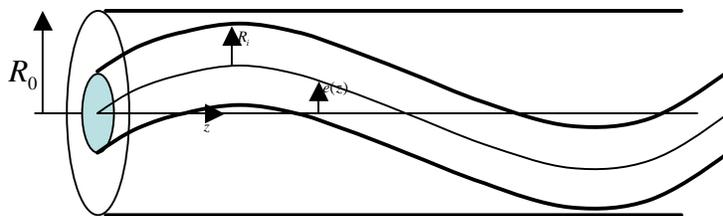
Figure 5: Sketch of annular space with the position of the center of the inner cylinder following a sinusoidal function.
