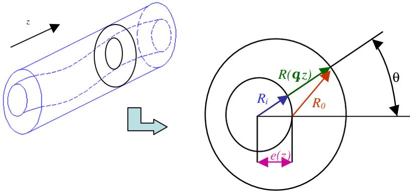
Figure 1: Configuration of annular space with eccentricity varying along the axial direction.
