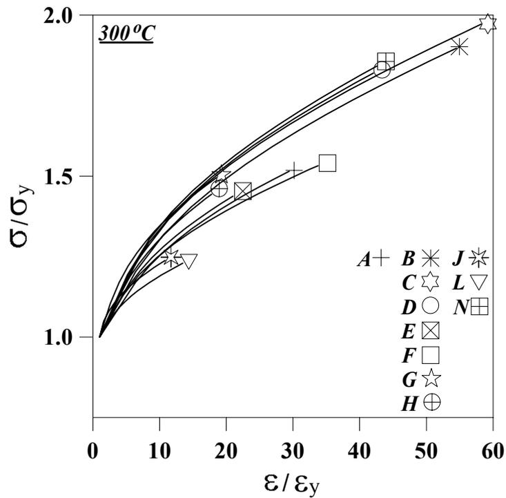
Figure 1. Parameterized power-law stress-strain curves determined according to Eq. (1).
