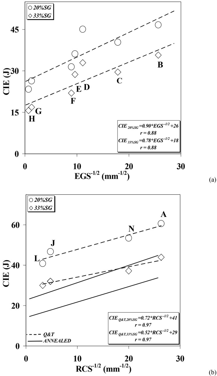
Figure 3. Hall-Petch dependence of CIE on RCS (or EGS), according to Eq. (4). (a) Annealed; (b) Q&T microstructures. In (b), results from annealed materials are drawn as baseline.
