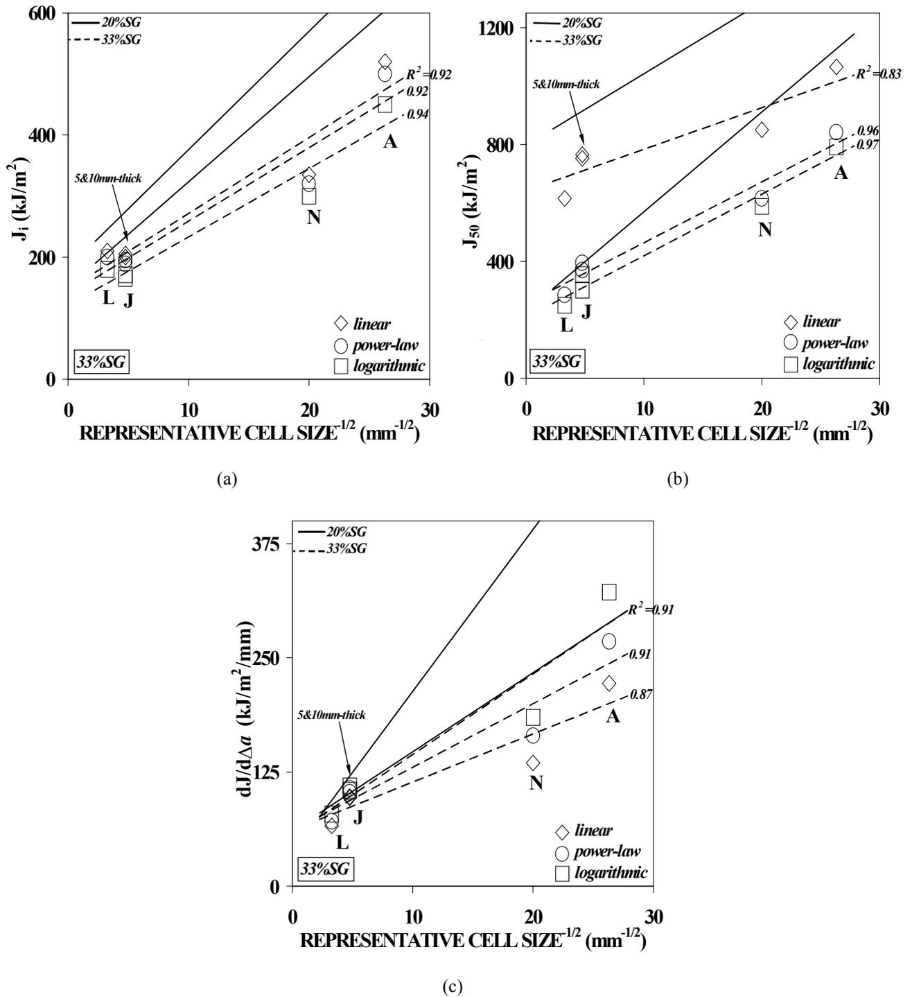
Figure 5. Relationships between J-parameters and equivalent cell size, according to Eq. (3). (a) Crack initiation  $J_i$ ; (b) Crack instability  $J_{50}$ , and (c) Rate of cracking resistance  $dJ/d\Delta a$ . Test specimens are 10mm-thick unless otherwise specified.
