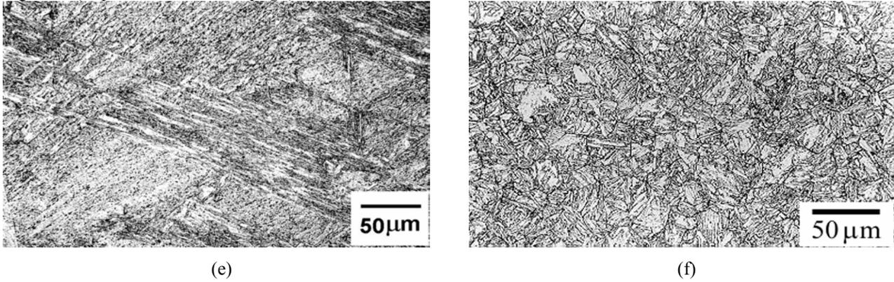
Figure 2. Light micrographs of materials tested: (a) I, (b) J (c) K, (d) L, (e) M, (f) N. Etched in Nital 2%.
