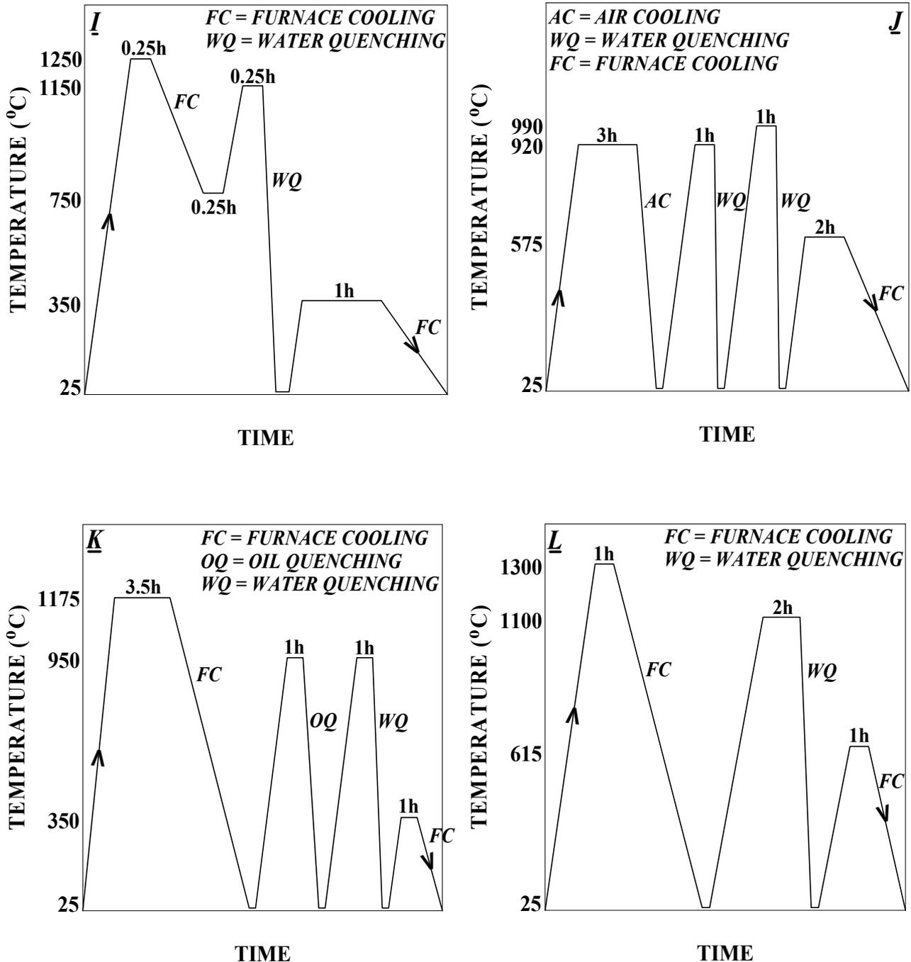
Figure 1. Schematic drawings of Q&T routes aimed at producing thermally embrittled microstructures (I-N) obtained from the original A508 steel (A). (Continued)
