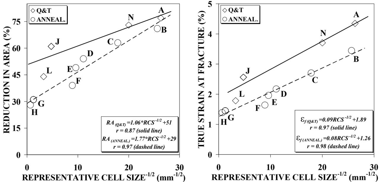
Figure 3. Hall-Petch relationship for the reduction in area (a) and true fracture strain (b) dependence on grain size for the materials tested. Previous results from Tarpani et al (2003) for annealed materials are also supplied.
