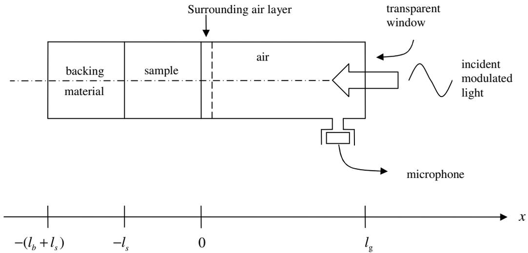
Figure 1 – Cross section of the photoacoustic cell.
