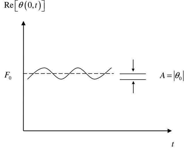
Figure 2 – Amplitude of the steady periodic temperature at  $x = 0$ .
