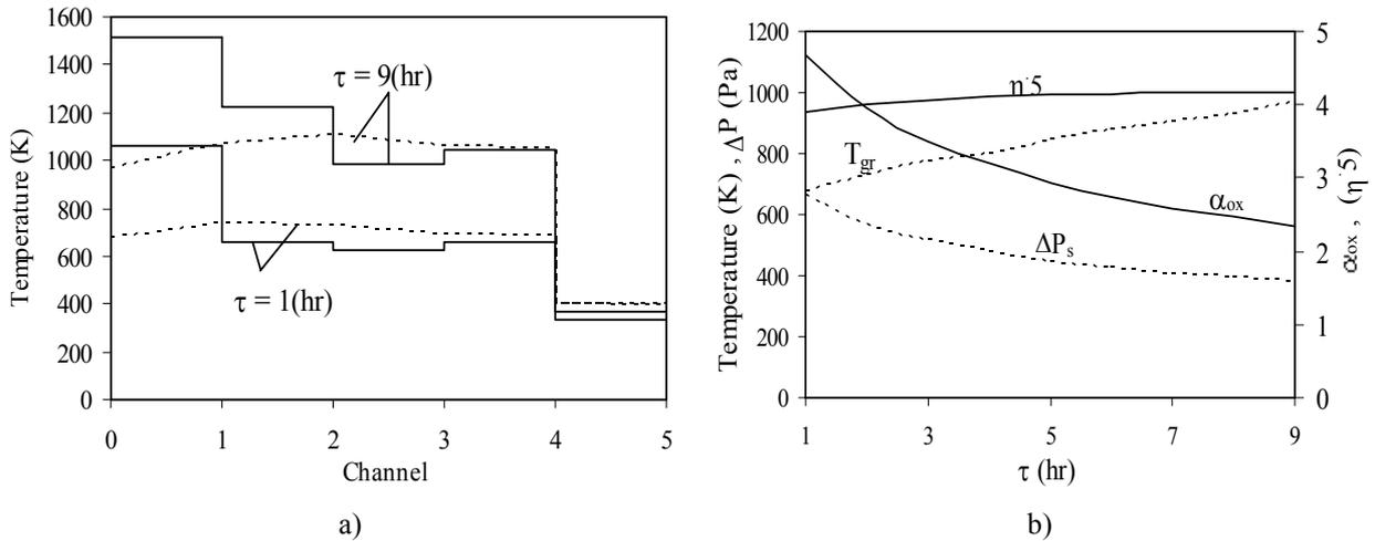
Figure 5. a) Distribution of  $T_k$  e  $T_{pi}$  along channels for  $\tau = 1\text{hr}$  and  $\tau = 9\text{hr}$  ( $T_{pi}$  — ;  $T_k$  - -); b) Evolution of furnace main characteristics
