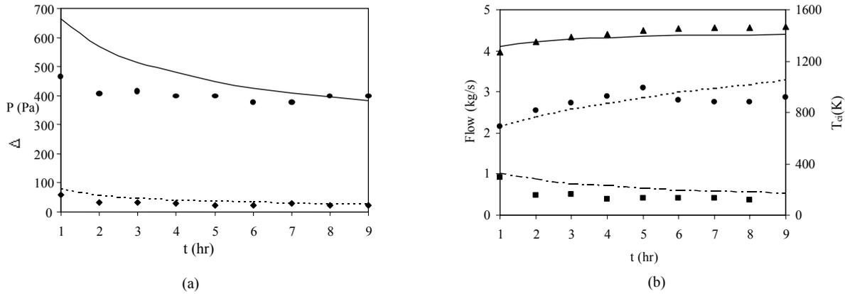
Figure 4. a) Pressure evolution:  $\Delta P_s$  (—) e  $\Delta P_{13}$  (- - -);  $\Delta P_{13}$  – pressure differences between atmosphere and end of channel 3c; ( $\bullet$ ,  $\blacklozenge$ ) – experimental data.; b) Mass flow rates  $G'_{pc}$  (---),  $G_s$  (—) and temperature  $T_{ci}$  (- - -) evolution
