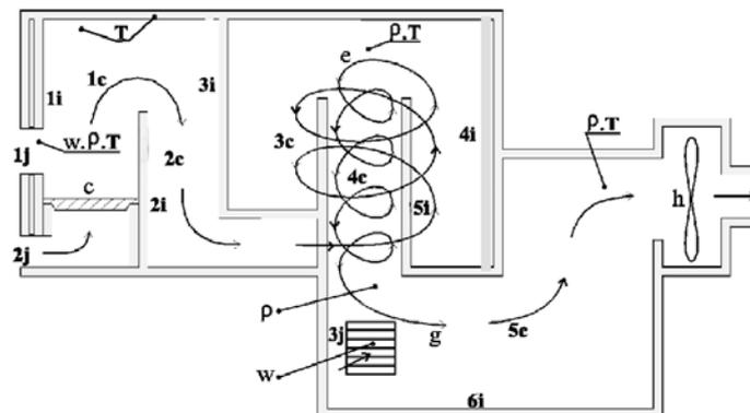
Figure 1. Scheme of industrial furnace: 1j, 2j, 3j - windows; c - grate; 1c, 2c, 3c, 4c, 5c – channels; 1i, 2i, 3i, 4i, 5i, 6i - walls; g - mixture zone; e - flows vortexes in cyclones; h – ventilator; P, T, W –points of measurement: pressure, temperature and velocity of flow, respectively.
