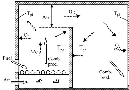
Figure 2. Heat radiation transfer scheme in channels 1c, 2c
