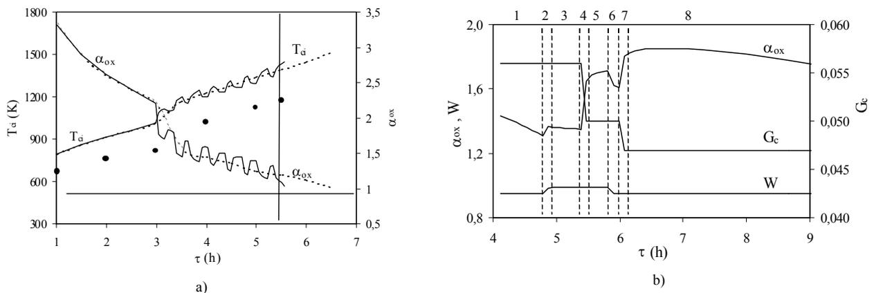
Figure 6. a) Evolutions  $T_{ci}$ ,  $\alpha'_{ox}$  in abnormal regime (• experiment; —, - - theory); b) Schedule off abnormal regime exit and the alteration of  $\alpha'_{ox}$  in this procedure.
