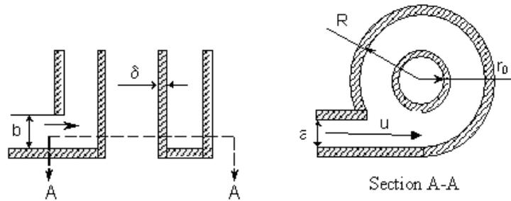
Figure 3. Scheme of furnace cyclone
