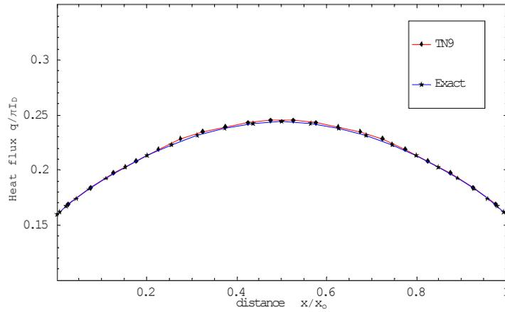
Fig. 5. Predicted heat flux at the bottom (cold) wall, comparison of  $T_9$  and exact solutions, Crosbie (1984), 20x20 grid, isotropic scattering case,  $\beta_{x/y}=1.0$ .
