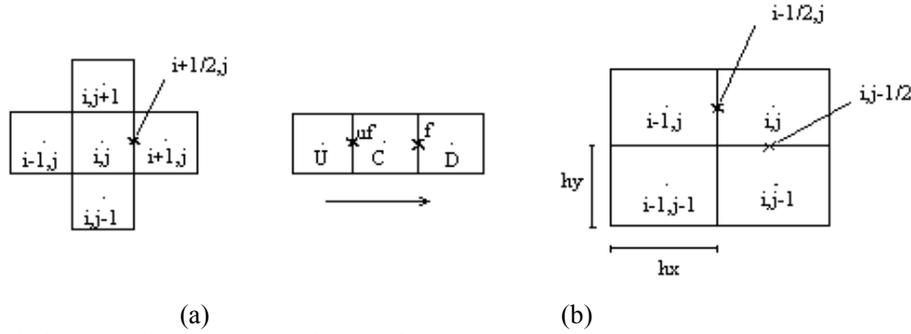
Figure 1. Interpolation stencil (a) CLAM scheme, (b) GM scheme
