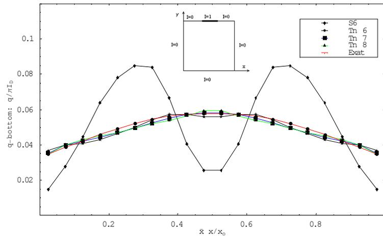
Fig. 6. Predicted heat flux at the bottom (cold) wall obtained for strip diffuse loading case,  $0.4 < x < 0.6$ , 20x20 grid, isotropic scattering,  $\beta_{x/y}=1.0$ . – Comparison with exact solution obtained by Crosbie (1984), and Ramankutte and Crosbie (1997).
