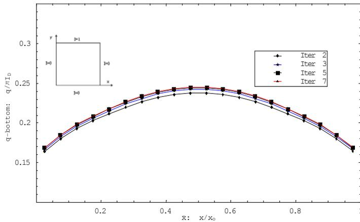
Fig. 2. Predicted heat flux at the bottom (cold) wall obtained by  $T_9$ ,  $20 \times 20$  grid, isotropic scattering case –Solution Convergence.
