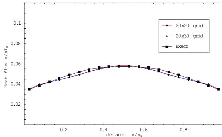
Fig 7. Predicted heat flux at the bottom (cold) wall obtained for strip diffuse loading case,  $0.4 < x < 0.6$ , isotropic scattering,  $\beta_{x/y}=1.0$ . – Comparison different grids with exact solution of Crosbie (1984) and Ramankutte and Crosbie (1997)
