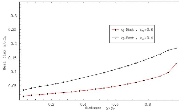
Fig 9. Heat Flux at west and east wall, different reflecting west and east walls case,  $\epsilon_w=0.8$ ,  $\epsilon_e=0.4$ ,  $\beta_{x/y}=1.0$ .
