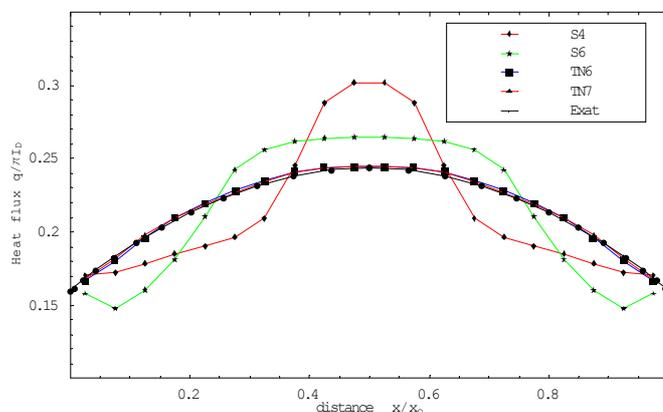
Fig. 4. Predicted heat flux at the bottom (cold) wall,  $S_N$  and  $T_N$  quadratures and exact solutions Crosbie (1984), Ramankutty and Crosbie (1997) comparison,  $20 \times 20$  grid, isotropic scattering case,  $\beta_{x/y} = 1.0$ .
