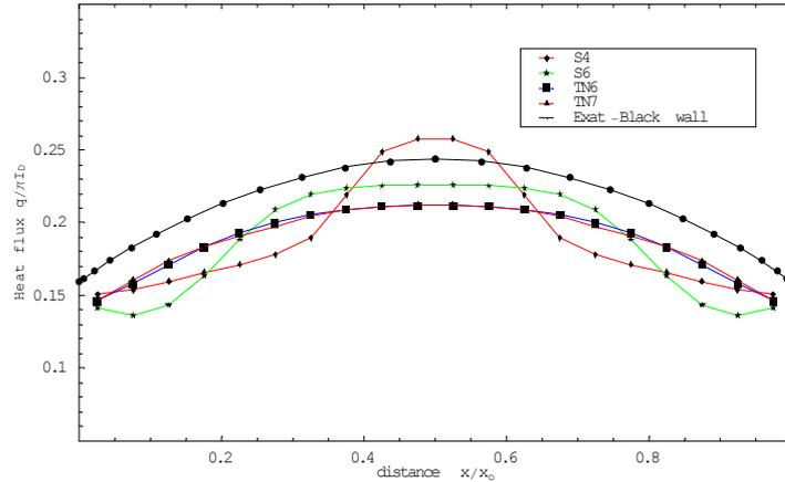
Fig. 8. Heat Flux at south cold wall, reflecting west and east walls case,  $\epsilon_w=0.8$ ,  $\epsilon_e=0.8$ ,  $\beta_{x/y}=1.0$ . Comparison of quadratures
