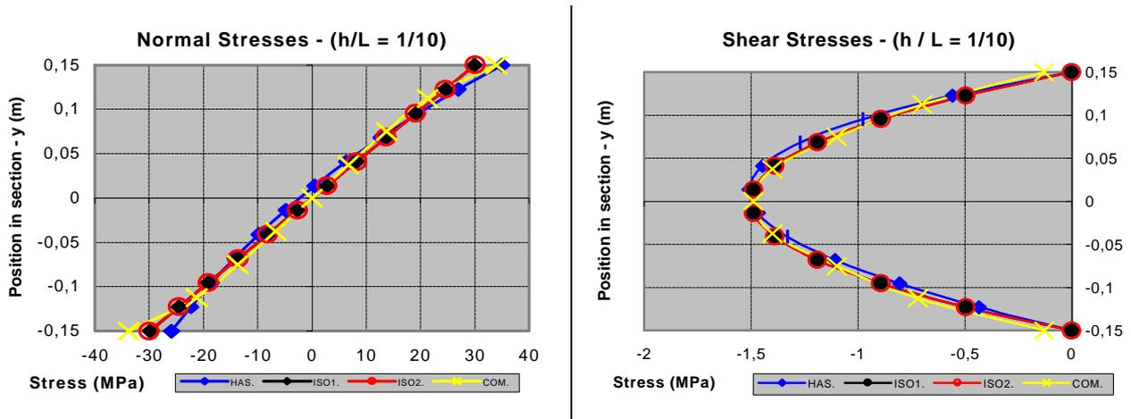
Figure 9. Normal and shear stresses in the laminated cantilever beam, relation ( $h / l = 1/10$ ), in two isotropic ones, considering the shear (ISO1) and not considering (ISO2), and in an orthotropic one.
