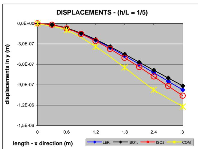
Figure 7. Displacement of a laminated cantilever beam, relation ( $h / l = 1/5$ ), of two isotropic ones, considering the shear (ISO1) and not considering (ISO2), and of an orthotropic one.
