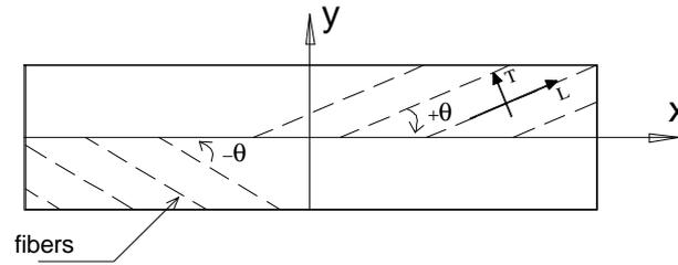
Figure 2. Angles of the fibers in the lamina.
