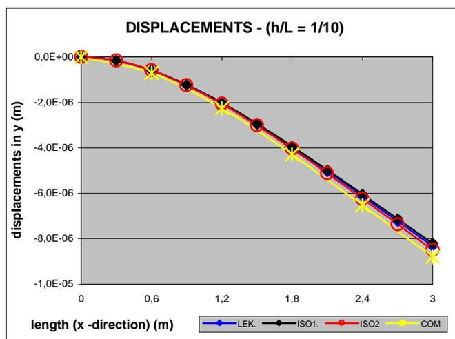
Figure 6. Displacement of a laminated cantilever beam, relation ( $h / l = 1/10$ ), of two isotropic ones, considering the shear (ISO1) and not considering (ISO2), and of an orthotropic one.
