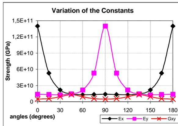
Figure 4. Values of the longitudinal elastic moduli of and the shear modulus.
