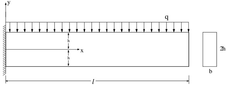
Figure 8. Cantilever beam, subjected to the uniformly distributed loads.
