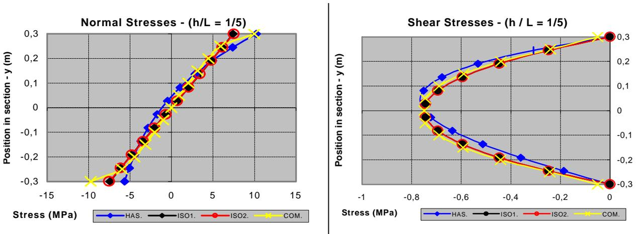
Figure 10. Normal and shear stresses in the laminated cantilever beam, relation ( $h / l = 1/5$ ), in two isotropic ones, considering the shear (ISO1) and not considering (ISO2), and in an orthotropic one.
