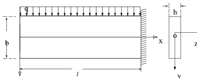
Figure 5. Cantilever beam subjected to uniformly distributed load.
