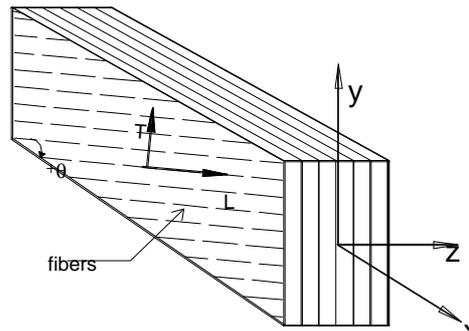
Figure 1. Laminated beam related to the systems geometric and local (of the fibers).
