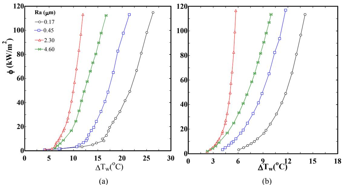
**Figure 3.** Boiling curves of refrigerant R-11 on copper surfaces. (a)  $p_r=0.011$ ; (b)  $p_r=0.092$ .
