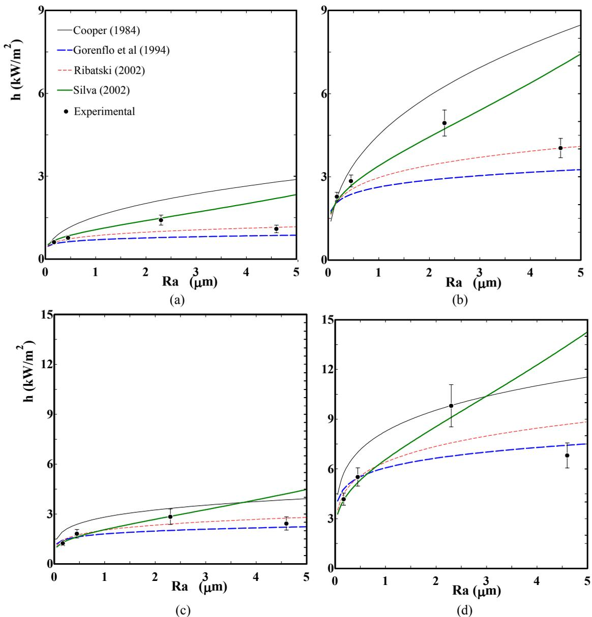
**Figure 4.** Heat transfer coefficient variation with surface roughness for nucleate boiling of refrigerant R-11 on copper surfaces. (a)  $p_r=0.011$  and  $\phi=10$   $\text{kW/m}^2$ ; (b)  $p_r=0.011$  and  $\phi=50$   $\text{kW/m}^2$ ; (c)  $p_r=0.092$  and  $\phi=10$   $\text{kW/m}^2$ ; (d)  $p_r=0.0921$  and  $\phi=50$   $\text{kW/m}^2$ .
