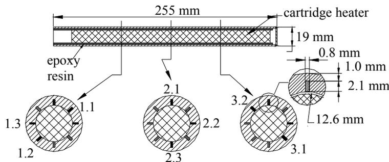
**Figure 2.** Longitudinal and transversal cut view of the test section showing the location of the surface thermocouples
