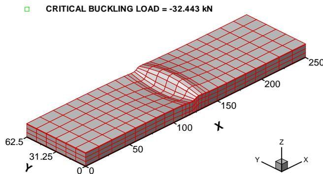
Figure 7 – Buckling of sandwich plate with discontinuous core.
