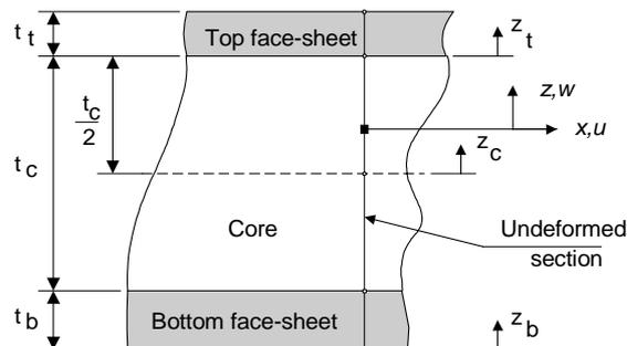
Figure 1 – Cross-section of the sandwich plate.
