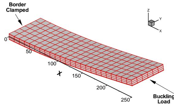
Figure 4 – Sandwich plate buckled with longitudinal in-plane compression.
