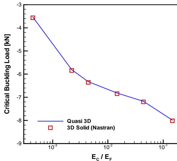
Figure 5 – Buckling load comparison for changing core stiffness.
