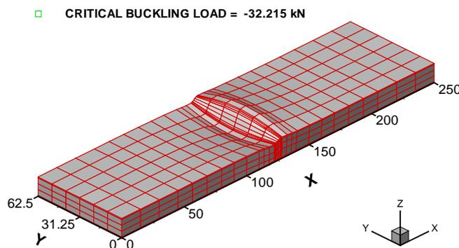
Figure 8 – Buckling of sandwich plate with discontinuous core (refined mesh).
