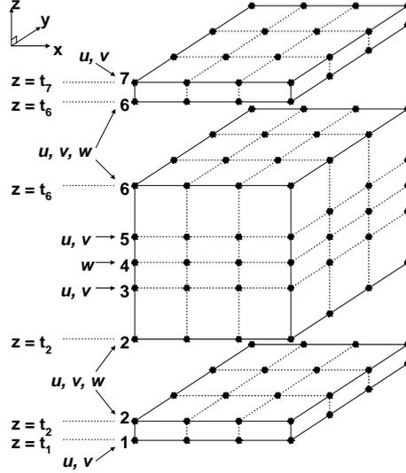
Figure 2 – Schematic of quasi 3D element (through-thickness degrees of freedom).
