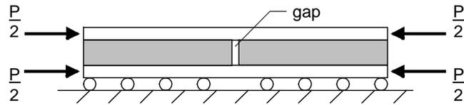
Figure 6 – Sandwich plate with discontinuous core.
