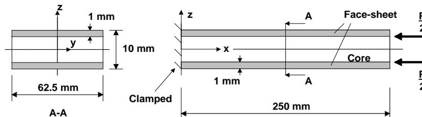
Figure 3 – Sandwich plate submitted to longitudinal in-plane compression.
