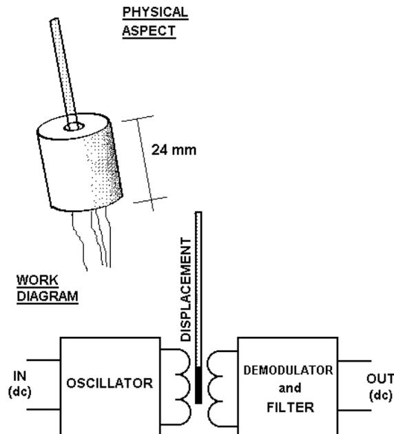
Figure 2. Transducer Displacement.
