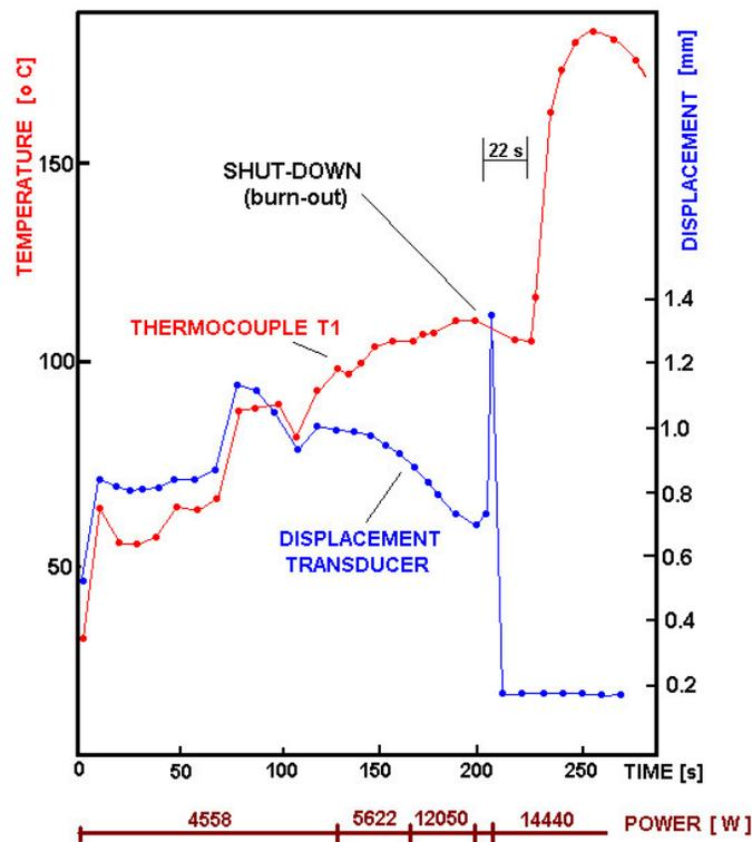
Figure 5 - Evolution of the temperature and of the sign of the transducer during the Test 14.
