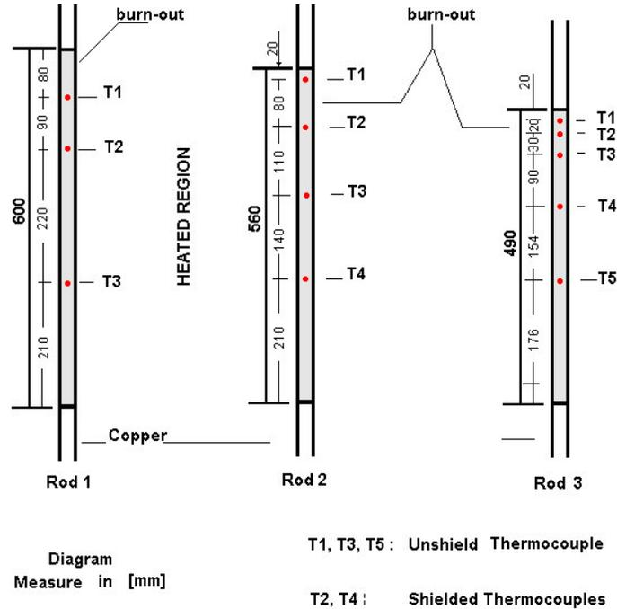
Figure 3 – Simulators rods.
